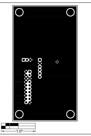
Figure 4. MAX1756 EV Kit PC Board Layout—Solder Side
