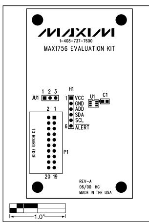
Figure 2. MAX1756 EV Kit Component Placement Guide— Component Side
