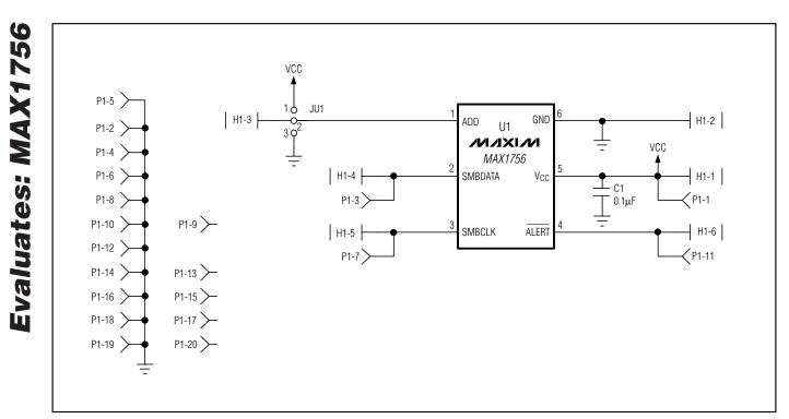
Figure 1. MAX1756 EV Kit Schematic
