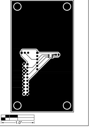
Figure 3. MAX1756 EV Kit PC Board Layout—Component Side
