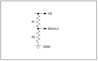
Figure 1. Setting the Input Undervoltage Lockout
