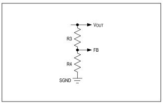
Figure 2: Adjusting Output Voltage
