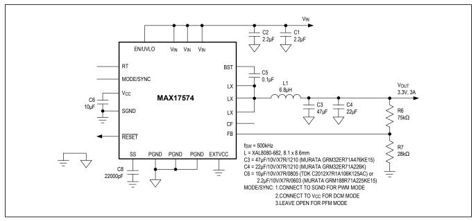
Figure 4. 3.3V Output Application Circuit
