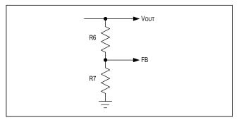
Figure 2. Adjusting Output Voltage
