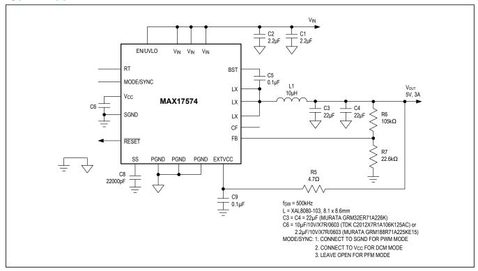
Figure 3. 5V Output Application Circuit
