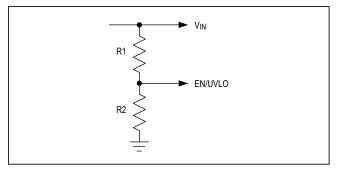
Figure 1. Setting the Input Undervoltage Lockout
