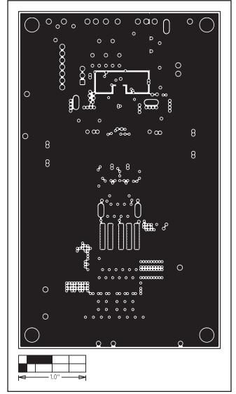
Figure 7. MAX17582 EV Kit PCB Layout—Internal Layer 5 (AGND/PGND Layer)
