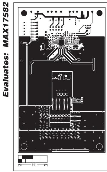
Figure 10. MAX17582 EV Kit PCB Layout—Solder Side
