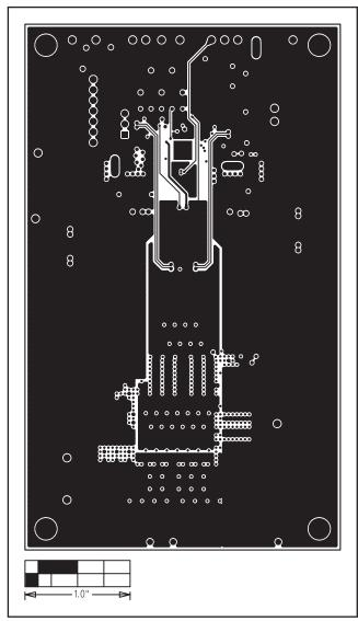
Figure 8. MAX17582 EV Kit PCB Layout—Internal Layer 6 (Signal Layer)
