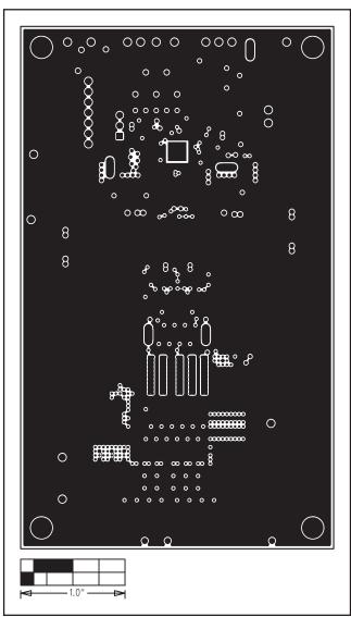
Figure 6. MAX17582 EV Kit PCB Layout—Internal Layer 4 (PGND Layer)
