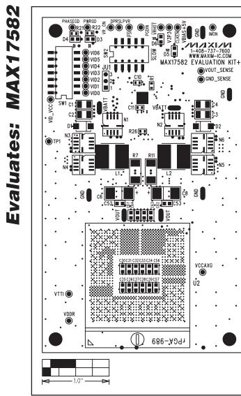
Figure 2. MAX17582 EV Kit Component Placement Guide— Component Side
