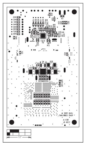
Figure 11. MAX17582 EV Kit Component Placement Guide—Solder Side
