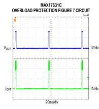
CONDITIONS: ADJUSTABLE 5V OUTPUT, PWM MODE, f<sub>SW</sub> = 850kHz
