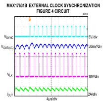
CONDITIONS: FIXED 5V OUTPUT, PWM MODE, 1.5A LOAD CURRENT f<sub>SW</sub> = 400kHz, EXTERNAL CLOCK FREQUENCY = 440kHz
