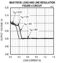
CONDITIONS: FIXED 5V OUTPUT, PFM MODE,  $\rm f_{SW}$  = 400kHz
