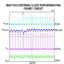
CONDITIONS: ADJUSTABLE 5V OUTPUT, PWM MODE, 1.5A LOAD CURRENT, f<sub>SW</sub> = 850kHz, EXTERNAL CLOCK FREQUENCY = 935kHz
