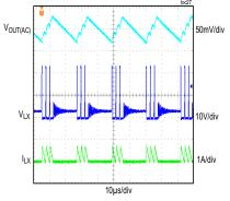
CONDITIONS: FIXED 3.3V OUTPUT, PFM MODE, 20mA LOAD, f<sub>SW</sub> = 400kHz
