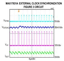
CONDITIONS: FIXED 3.3V OUTPUT, PWM MODE, 1.5A LOAD CURRENT  $\rm f_{SW}$  = 400kHz, EXTERNAL CLOCK FREQUENCY = 440kHz
