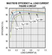
CONDITIONS: FIXED 5V OUTPUT, PWM MODE, f<sub>SW</sub> = 400kHz
