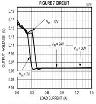
CONDITIONS: ADJUSTABLE 5V OUTPUT, PFM MODE, f<sub>SW</sub> = 850kHz
