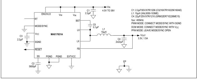
Figure 3. Fixed 3.3V Output with 400kHz Switching Frequency
