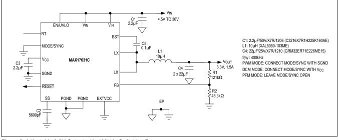
Figure 5. Adjustable 3.3V Output with 400kHz Switching Frequency
