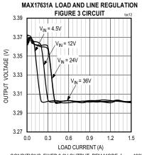
CONDITIONS: FIXED 3.3V OUTPUT, PFM MODE, f<sub>SW</sub> = 400kHz
