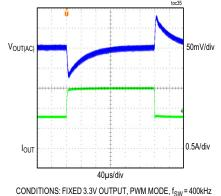
MAX17631A LOAD TRANSIENT BETWEEN 40mA AND 0.75A FIGURE 3 CIRCUIT
