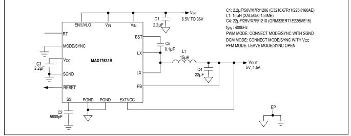
Figure 4. Fixed 5V Output with 400kHz Switching Frequency
