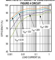
CONDITIONS: FIXED 5V OUTPUT, PFM MODE,  $\rm f_{SW}$  = 400kHz
