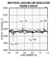
CONDITIONS: FIXED 5V OUTPUT, DCM MODE, f<sub>SW</sub> = 400kHz
