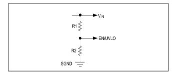
Figure 1. Setting the Input Undervoltage Lockout
