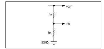
Figure 2. Setting the Output Voltage
