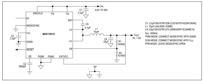
Figure 6. Adjustable 5V Output with 400kHz Switching Frequency
