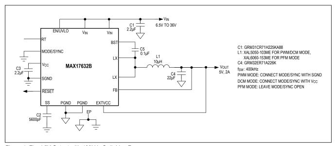
Figure 4. Fixed 5V Output with 400kHz Switching Frequency
