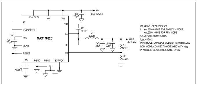
Figure 5. Adjustable 3.3V Output with 400kHz Switching Frequency
