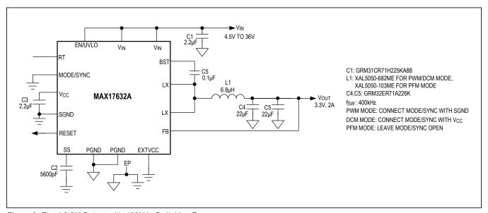
Figure 3. Fixed 3.3V Output with 400kHz Switching Frequency
