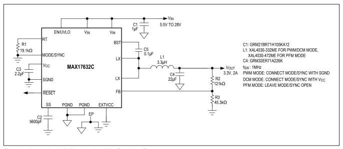
Figure 7. Adjustable 3.3V Output with 1MHz Switching Frequency
