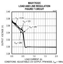
$(V_{EN/UVLO} = V_{IN} = 24V, V_{SGND} = V_{PGND} = 0V, C_{VCC} = 2.2\mu\text{F}, C_{BST} = 0.1\mu\text{F}, C_{SS} = 5600\text{pF}, T_{A} = -40^{\circ}\text{C} \text{ to } +125^{\circ}\text{C}, \text{ unless otherwise noted.}$
