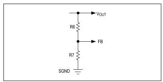
Figure 2. Setting the Output Voltage
