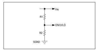
Figure 1. Setting the Input Undervoltage Lockout
