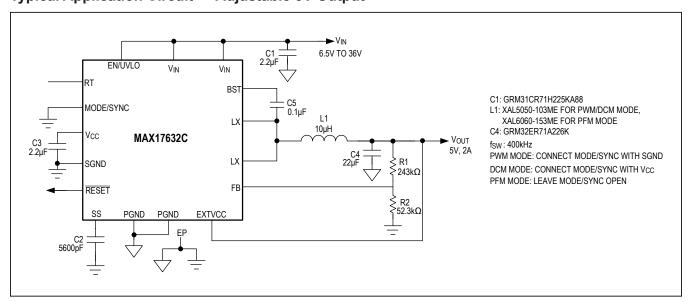
Figure 6. Adjustable 5V Output with 400kHz Switching Frequency
