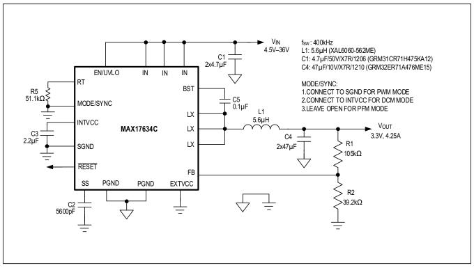
Figure 3. Adjustable 3.3V Output with 400kHz Switching Frequency
