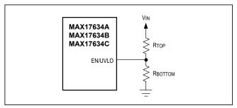
Figure 1. Setting the Input Undervoltage Lockout
