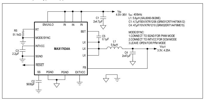
Figure 5. Fixed 3.3V Output with 400kHz Switching Frequency
