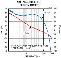
CONDITIONS: ADJUSTABLE 5V OUTPUT, 4.25A LOAD, PWM MODE
