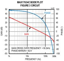
CONDITIONS: ADJUSTABLE 3.3V OUTPUT, 4.25A LOAD, PWM MODE
