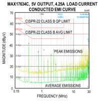
CONDITIONS: MEASURED ON THE MAX17634CEVKIT WITH L2 = 22µH, C12 = C13 = 2.2µF/50V/X7R/1206, C14 = C19 = 4.7µF/50V/X7R/1210
