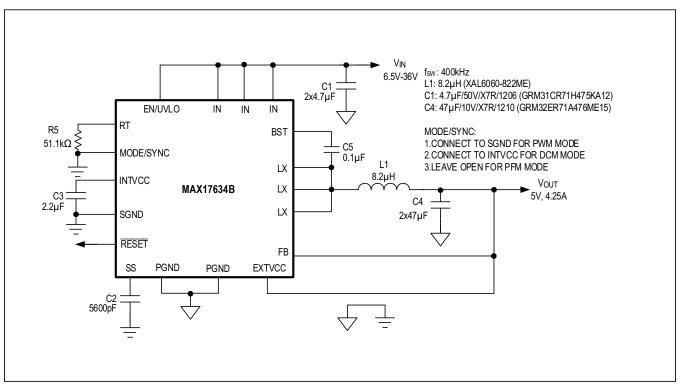
Figure 6. Fixed 5V Output with 400kHz Switching Frequency
