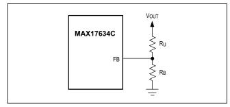
Figure 2. Setting the Output Voltage
