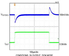
CONDITIONS: 5V OUTPUT, DCM MODE, C4 =  $47\mu F/10V/X7R/1210$ , R3 =  $182k\Omega$ , R4 =  $24.9k\Omega$
