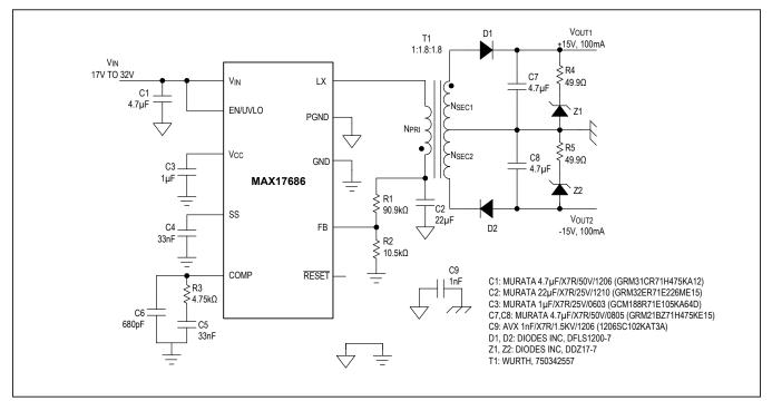
Figure 10. ±15V, 100mA Isolated Output Application Circuit
