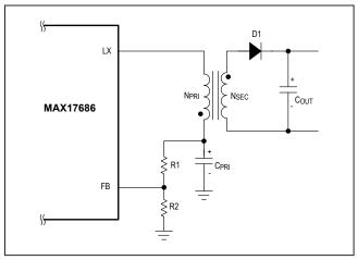
Figure 5. Adjusting the Primary Output Voltage
