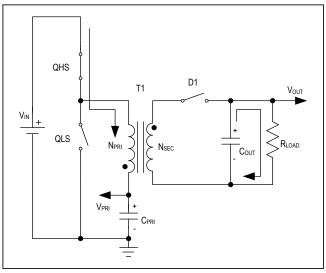
Figure 2. On-Period Equivalent Circuit
