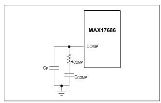
Figure 7. External Compensation Network
