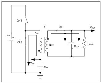
Figure 3. Off-Period Equivalent Circuit
