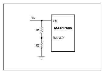
Figure 6. Adjustable EN/UVLO Network
