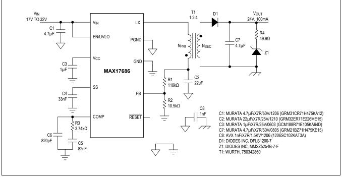
Figure 9. 24V, 100mA Isolated Output Application Circuit
