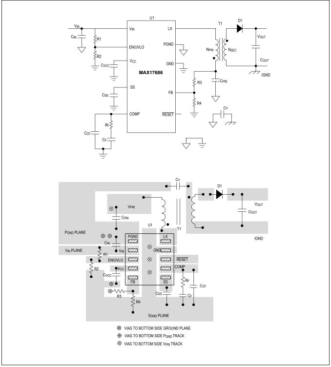
Figure 8. Recommended Component Placement
