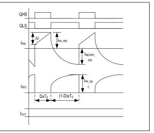
Figure 4. Iso-Buck Operating Waveforms
