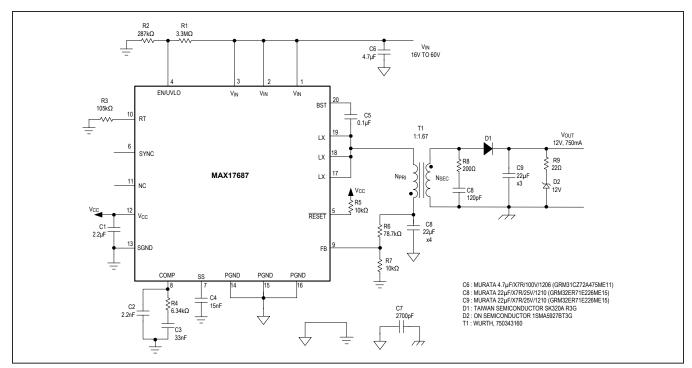
Figure 9: 12V, 750mA Isolated Output Application Circuit -2
