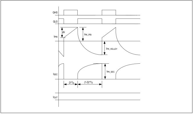
Figure 4. Iso-Buck Operating Waveforms
