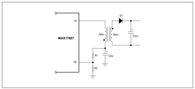
Figure 5. Adjusting Primary Output Voltage
