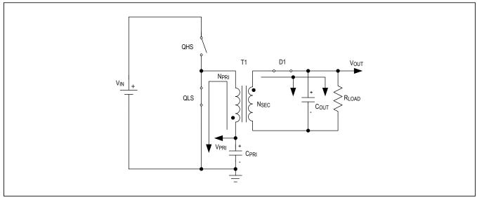
Figure 3. Off Period Equivalent Circuit
