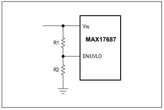
Figure 6. Setting the Input Undervoltage Lockout
