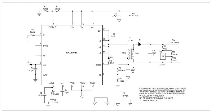
Figure 8: 12V, 750mA Isolated Output Application Circuit -1
