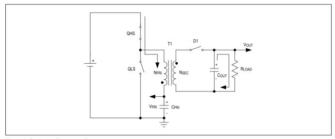
Figure 2. On Period Equivalent Circuit
