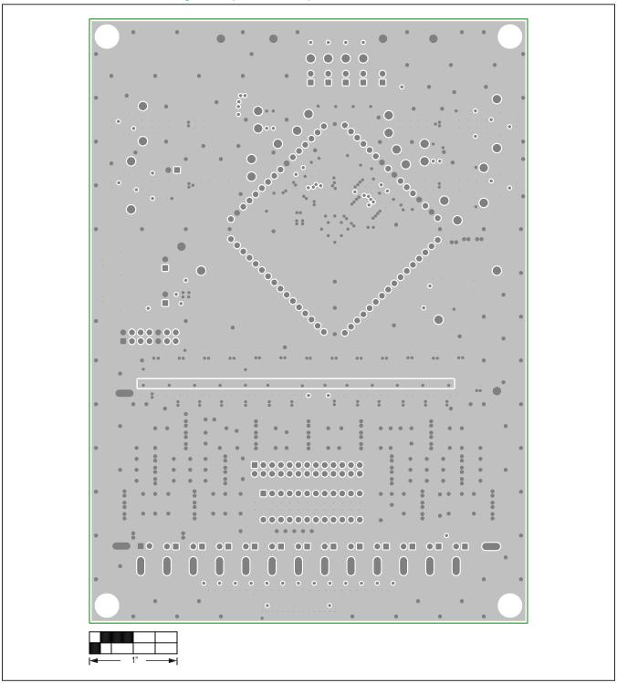
Figure 26. MAX17823 EV Kit PCB Layer Two Metal
