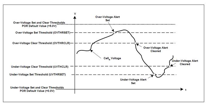
Figure 19. Programmable OV and UV Thresholds Diagram
