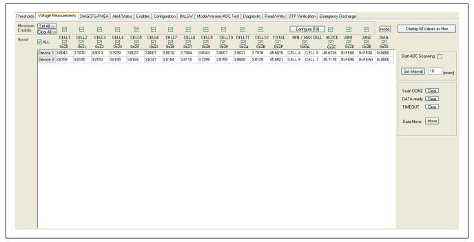
Figure 9. MAX17823 Evaluation Kit Software (Voltage Measurements Tab)
