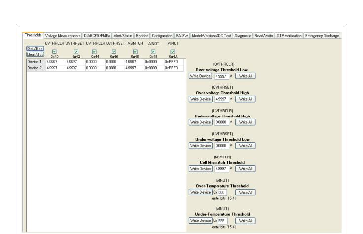
Figure 8. MAX17823 Evaluation Kit Software (Thresholds Tab)
