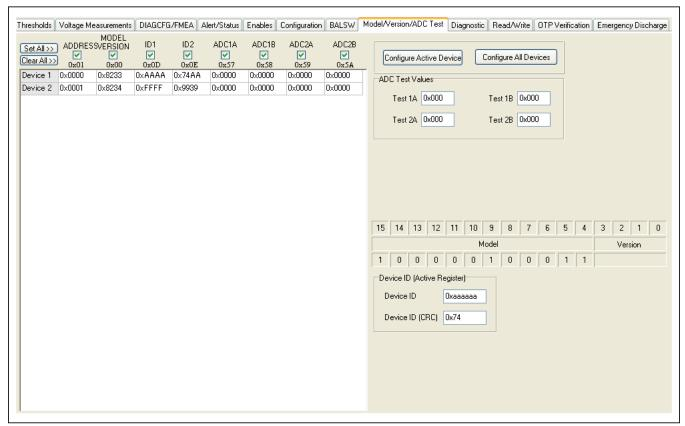
Figure 15. MAX17823 Evaluation Kit Software (Model/Version/ADC Test Tab)
