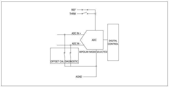
Figure 96. Offset-Calibration Diagnostic
