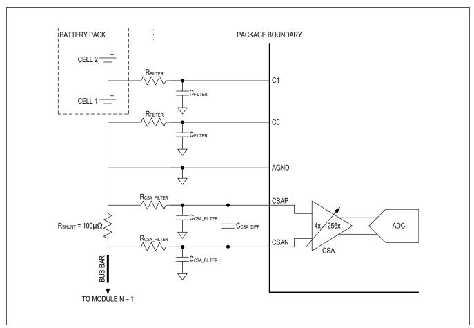
Figure 12. Current Measurement Configuration
