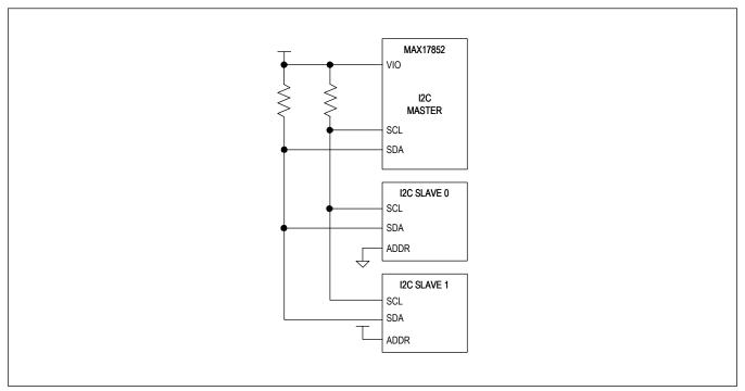
Figure 75. I<sup>2</sup>C Device Connection
