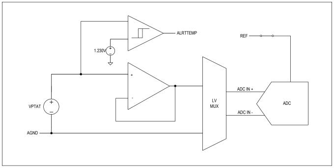
Figure 89. Die Temperature Measurement
