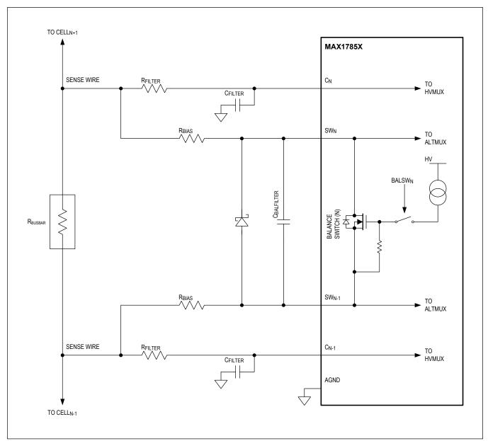
Figure 7. Bus-Bar Switch Configuration
