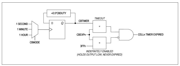
Figure 47. Cell-Balancing Expiration Timer
