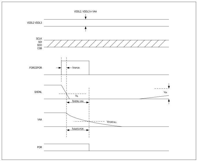
Figure 22. Power-On and Shutdown Timing (SPI Control)
