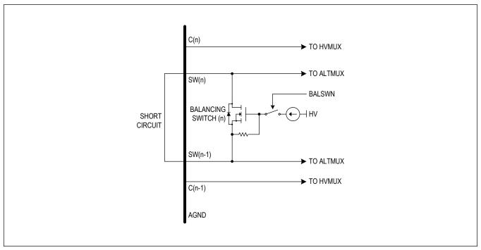
Figure 102. Balancing Switch Short
