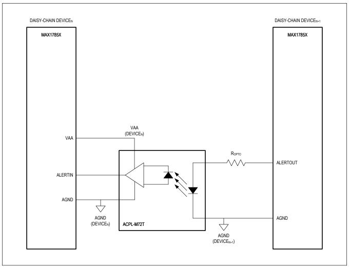
Figure 128. Single-End ALERT Interface in UART mode
