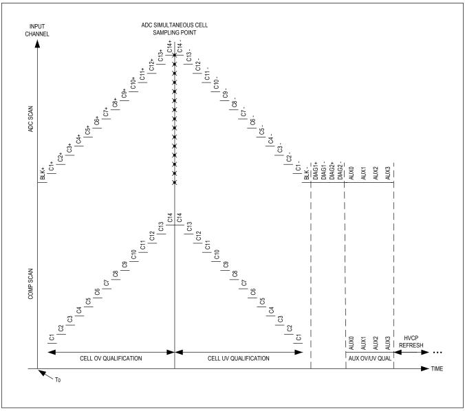
Figure 32. Simultaneous ADC+COMP Scan With Oversampling
