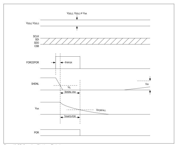
Figure 18. SPI Operation (Shutdown Timing)
