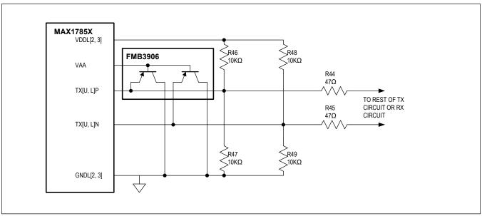
Figure 120. High-Z Idle Mode Application Circuit
