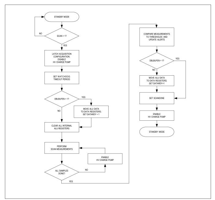
Figure 36. Acquisition-Mode Flowchart
