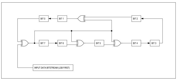
Figure 132. PEC CRC Calculation
