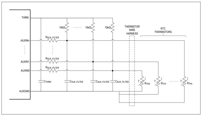
Figure 9. Auxiliary Application Circuit
