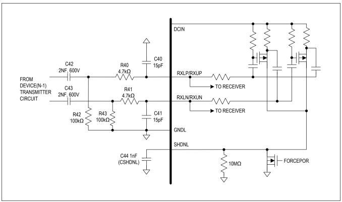
Figure 62. SHDNL Charge Pump
