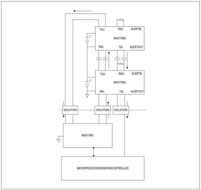
Figure 56. Single UART with Differential Alert Interface
