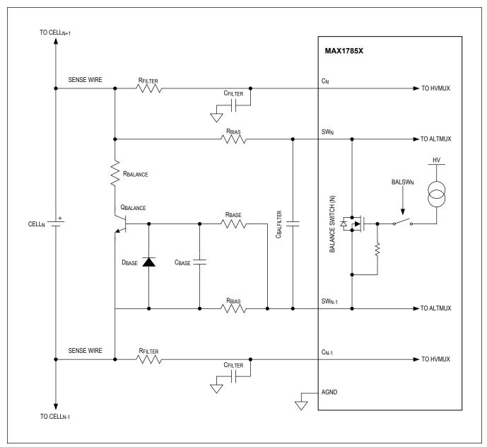
Figure 118. External Cell Balancing-BJT
