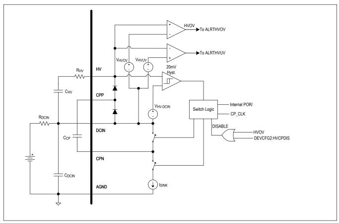
Figure 88. HV Charge Pump
