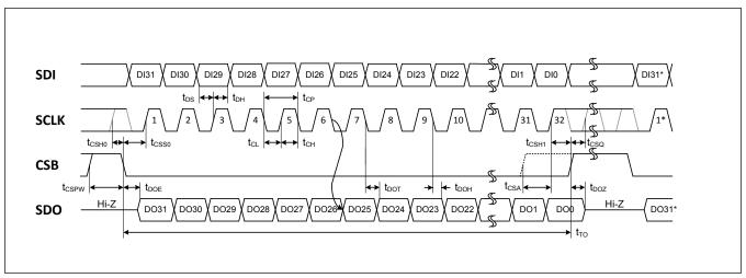
Figure 68. SPI Timing Diagram
