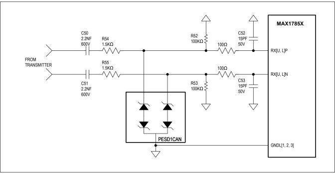
Figure 122. External ESD Protection for UART RX Ports
