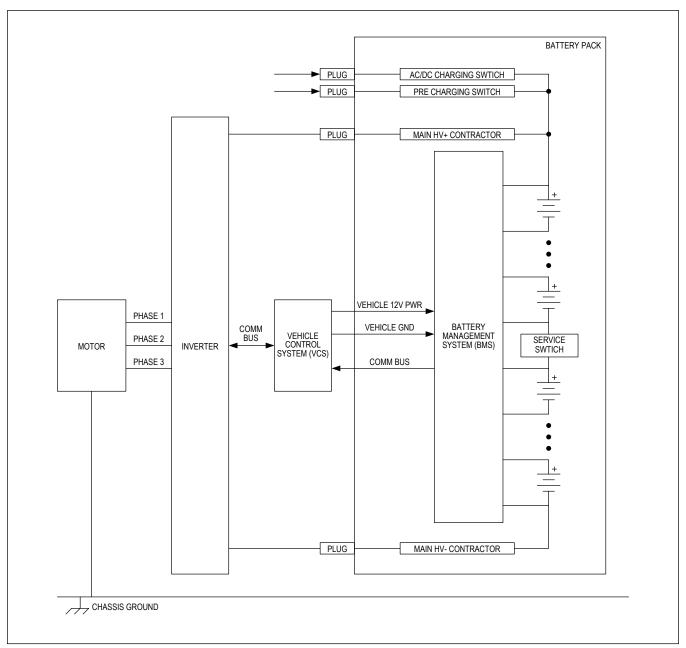
Figure 111. Electric Vehicle System
