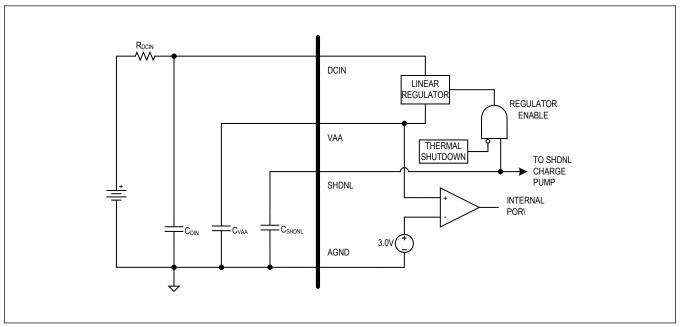
Figure 87. Low-Voltage Regulator and Thermal-Shutdown Circuit
