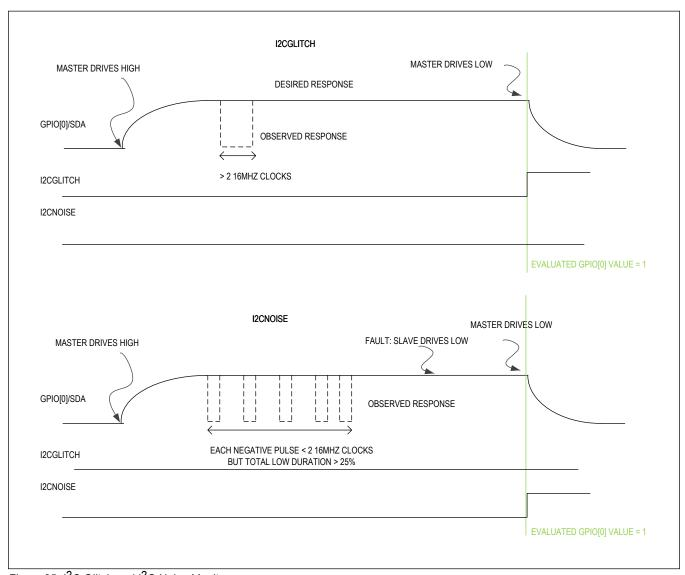
Figure 85. I<sup>2</sup>C Glitch and I<sup>2</sup>C Noise Monitor
