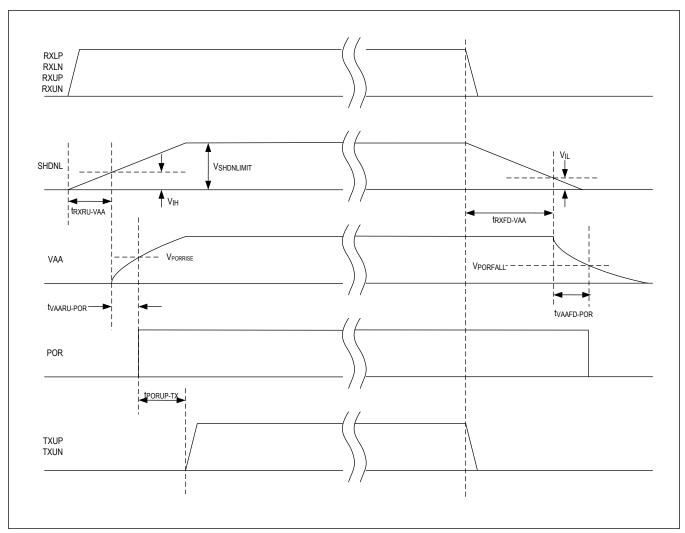
Figure 19. Power-On Timing (UART-Communication Control)
