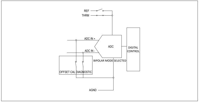
Figure 97. THRM Offset -Calibration Diagnostic
