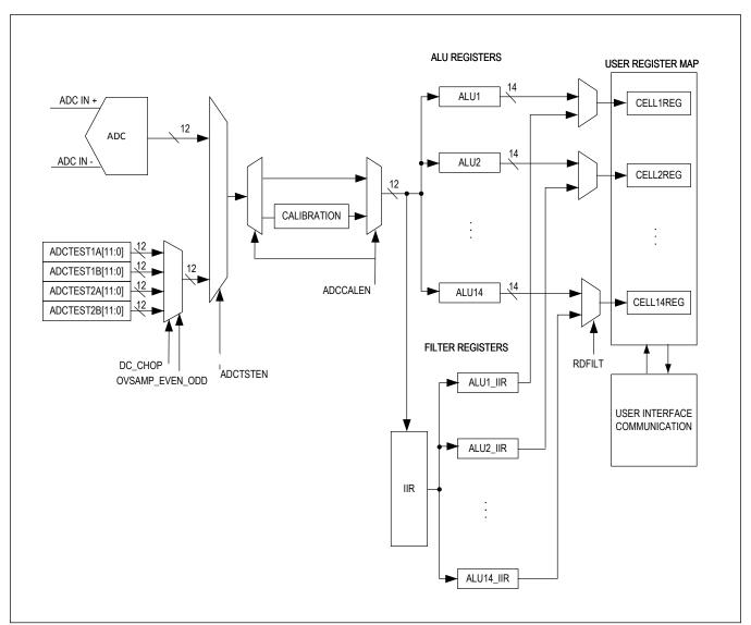
Figure 37. Data-Flow Diagram
