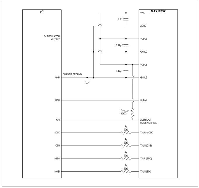
Figure 127. 3.3V SPI Supply from Device V<sub>AA</sub> LDO
