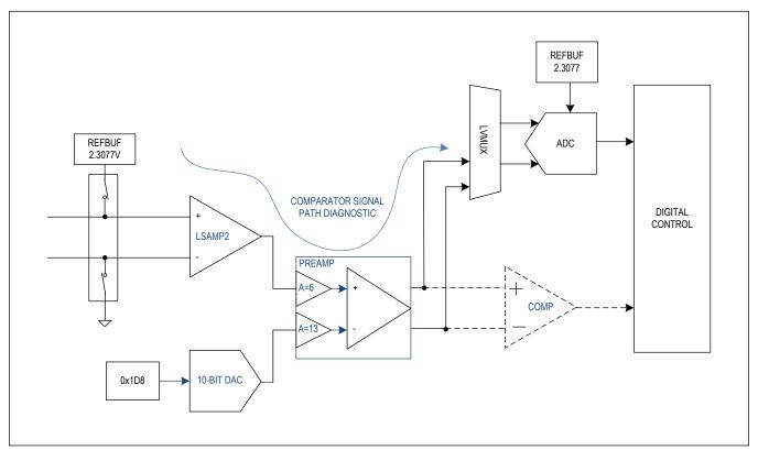
Figure 92. Comparator Signal Path to ADC
