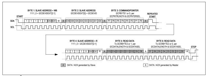
Figure 79. I<sup>2</sup>C Combined Format Read Mode Transaction Example -- 10-Bit Address, I2C10BIT = 1, I2CRFMT = 1
