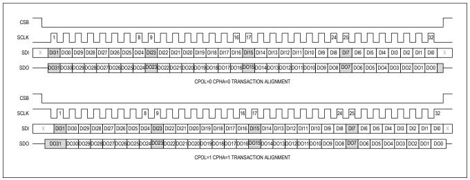
Figure 70. SPI Supported Transaction Alignments
