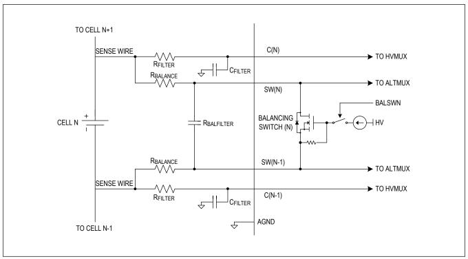
Figure 53. Internal Cell-Balancing Switches
