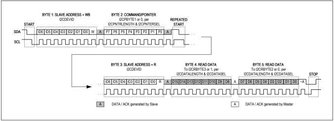
Figure 80. I<sup>2</sup>C Combined Format Read Mode Transaction Example -- 7-Bit Address, I2C10BIT = 0, I2CRFMT = 1
