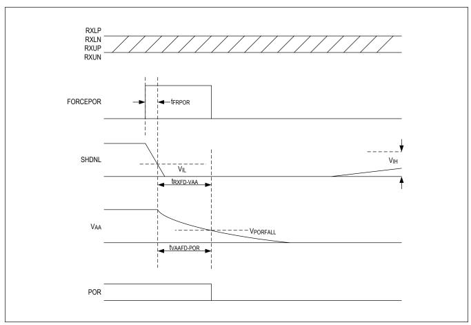
Figure 17. UART Operation (Shutdown Timing)
