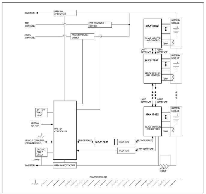
Figure 113. Figure: Daisy-Chain System with CSA
