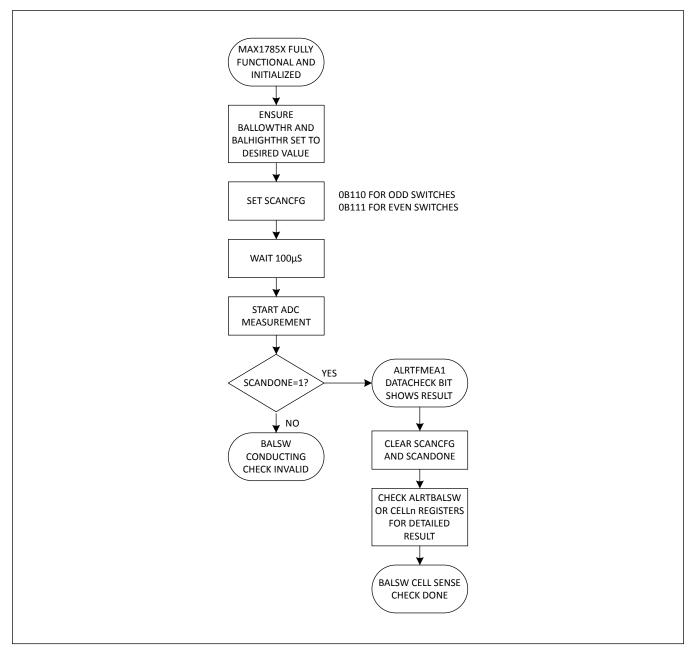
Figure 105. Sense-Wire Open-Diagnostic Flow
