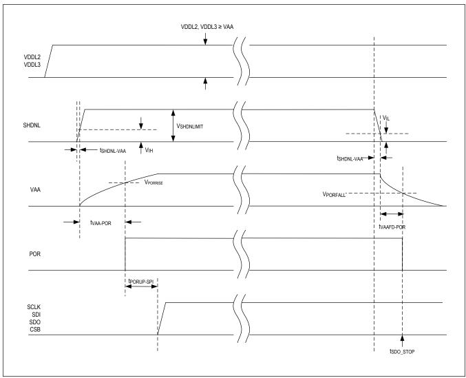
Figure 20. Power-On Timing (SPI Directed Control)
