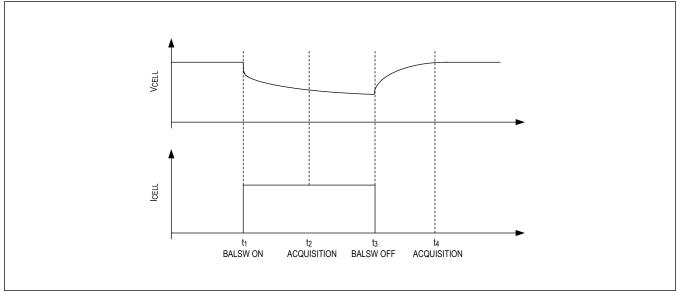
Figure 44. AUTOBALSWDIS Measurement Settling
