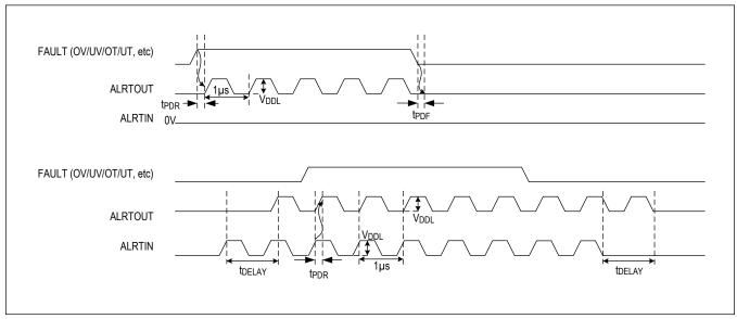
Figure 86. UART Mode Alert Detection Timing Diagram
