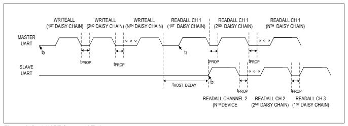
Figure 59. Dual-UART Command Timing
