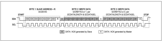
Figure 82. I<sup>2</sup>C Normal Format Read Mode Transaction Example -- 7-Bit Address, I2C10BIT = 0, I2CRFMT = 0
