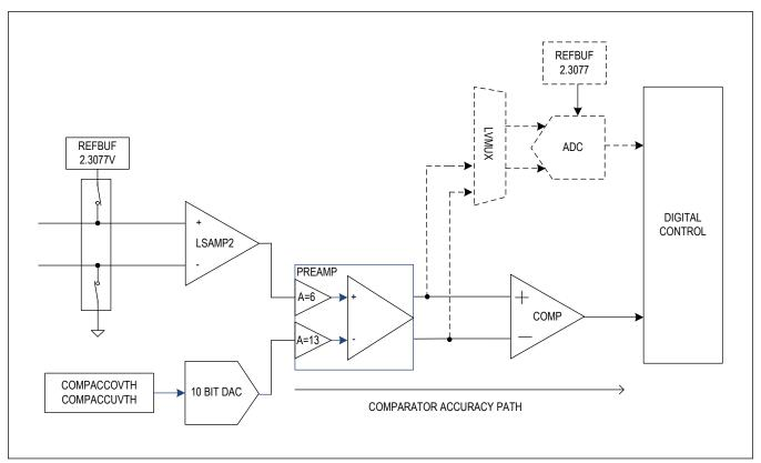
Figure 93. Comparator Accuracy Diagnostic Path
