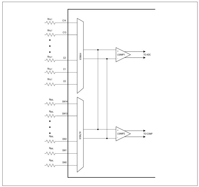
Figure 6. Cell Signal Path
