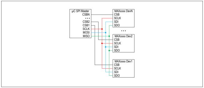
Figure 69. SPI Device Connection
