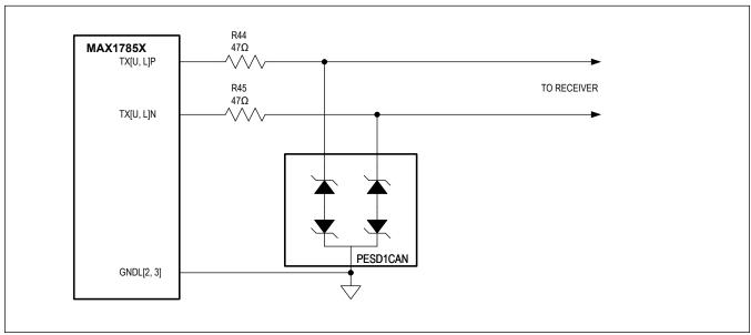
Figure 121. External ESD Protection for UART TX Ports
