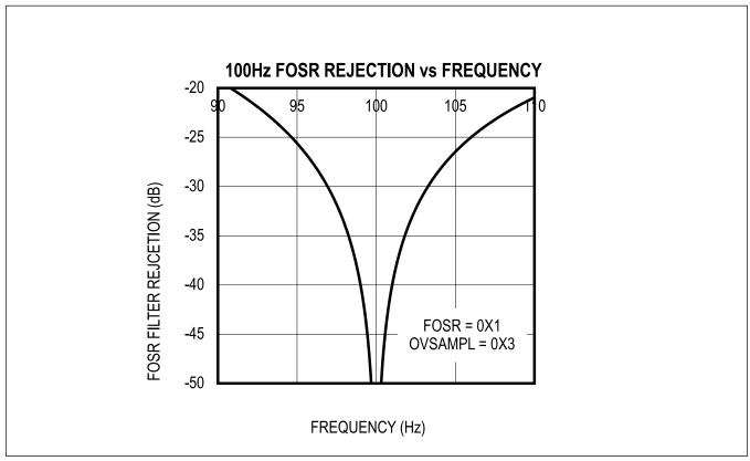
Figure 34. 100Hz Notch Filter
