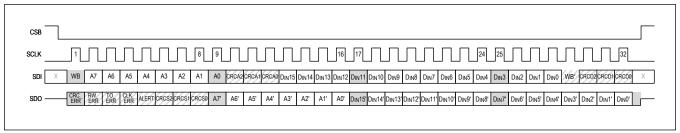
Figure 71. SPI Write-Mode Transaction Format
