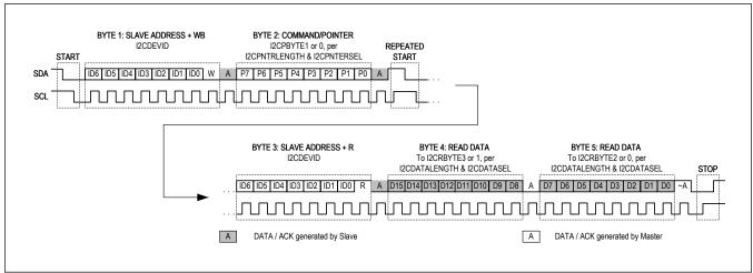
Figure 78. I<sup>2</sup>C Combined Format Read Mode Transaction Example -- 7-Bit Address, I2C10BIT = 0, I2CRFMT = 1
