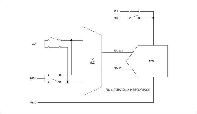
Figure 99. ADC Zero-Scale Diagnostic
