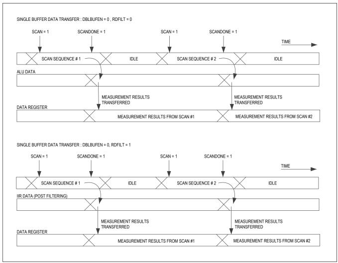
Figure 40. Single-Buffer Data Transfer
