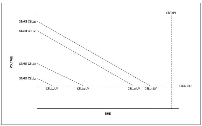
Figure 48. Cell-Balancing UV Threshold Crossing
