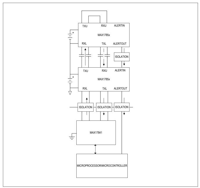
Figure 55. Single UART with External Loopback
