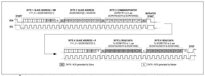
Figure 81. I<sup>2</sup>C Combined Format Read Mode Transaction Example -- 10-Bit Address, I2C10BIT = 1, I2CRFMT = 1
