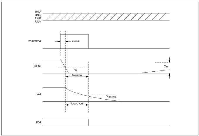
Figure 21. Power-On and Shutdown Timing (UART Control)
