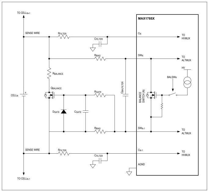
Figure 117. External Balancing-FET
