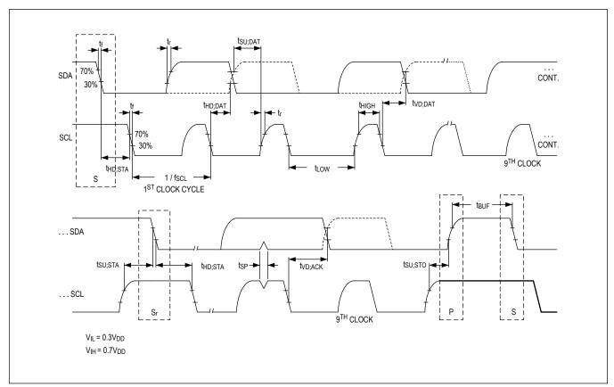
Figure 74. Standard I<sup>2</sup>C BUS Timing Diagram
