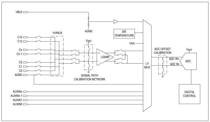
Figure 33. On Demand Calibration Block Diagram
