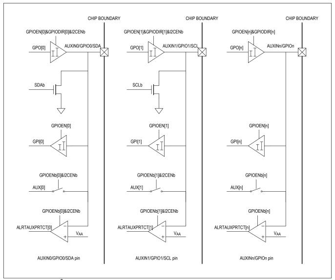
Figure 11. AUX/GPIO/I<sup>2</sup>C Pin Connections
