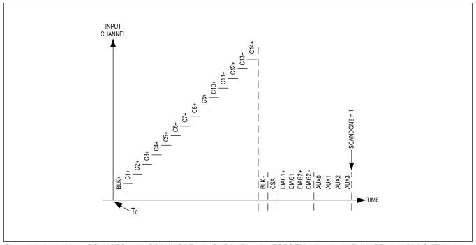
Figure 28. Acquisition - SCANCFG = 0h, SCANMODE = 1, OVSAMPL = 0h, TOPCELL1/2 = 14, ALTMUXSEL = 1, BLOCKEN = 1, CSAEN = 1, DIAGSEL1 > 0h, DIAGSEL2 > 0h, AUXEN = Fh
