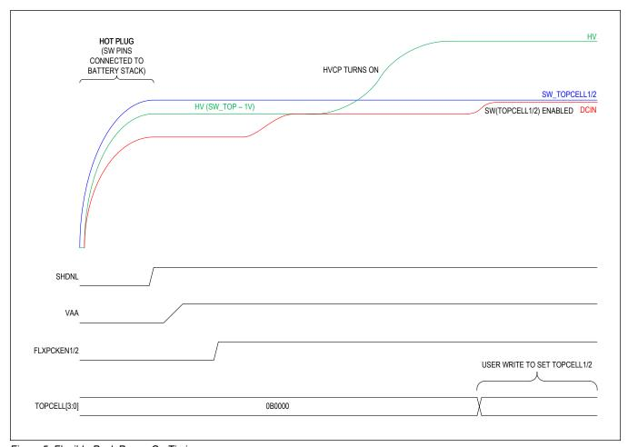
Figure 5. Flexible-Pack Power-On Timing
