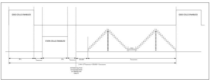
Figure 46. Auto Even Odd Cell Balancing with UV Detection, ADC with OVSAMPL
