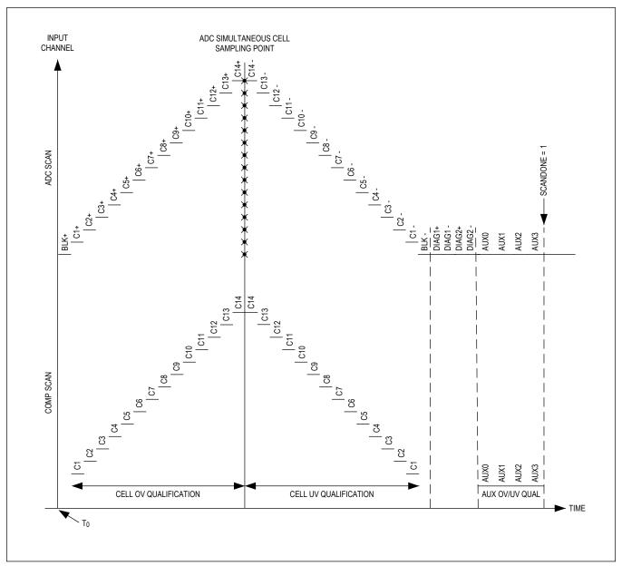
Figure 31. Simultaneous ADC+COMP Scan Mode
