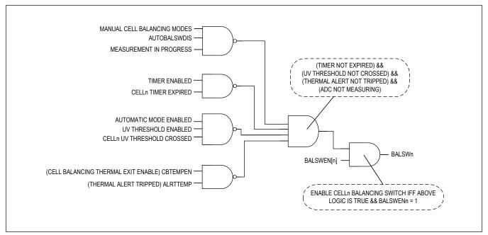
Figure 51. Cell-Balancing Stop Control
