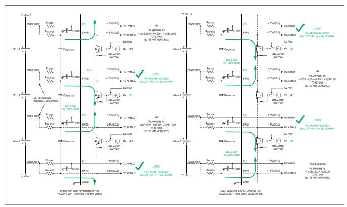
Figure 106. Cell Sense-Wire Open-Diagnostic Operations - (Normal Operation)
