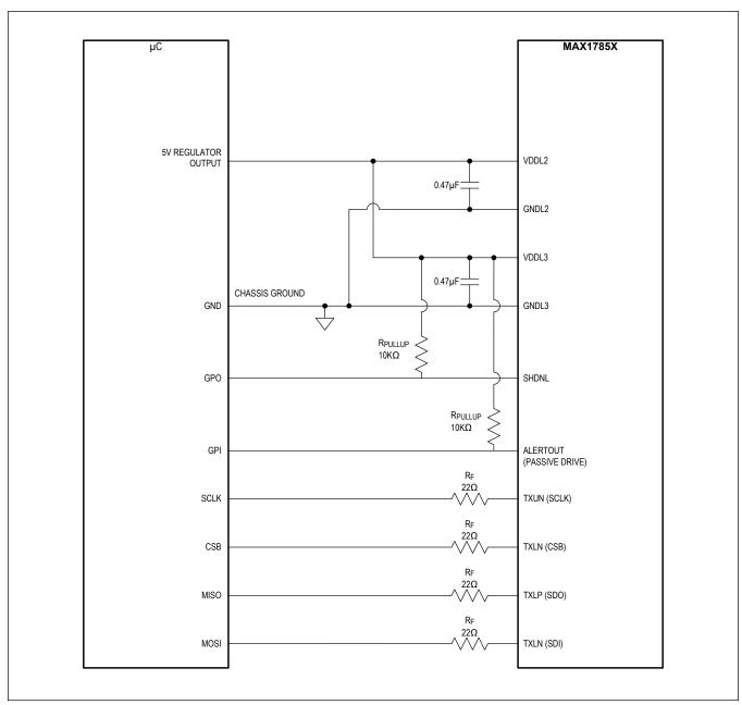
Figure 126. 5V SPI Supply from System
