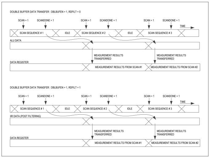
Figure 41. Double-Buffer Data Transfer
