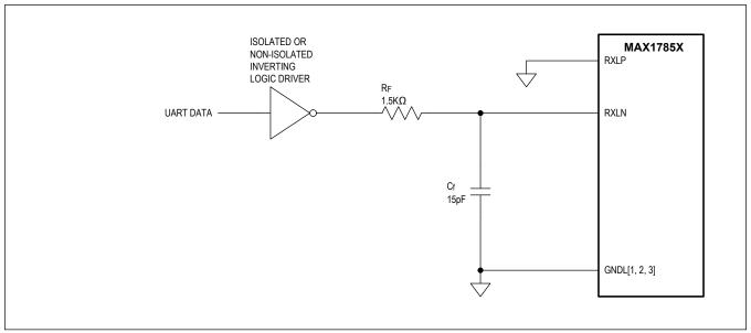
Figure 123. Application Circuit for Single-Ended UART Mode
