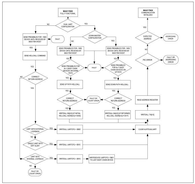
Figure 131. Device Initialization Sequence
