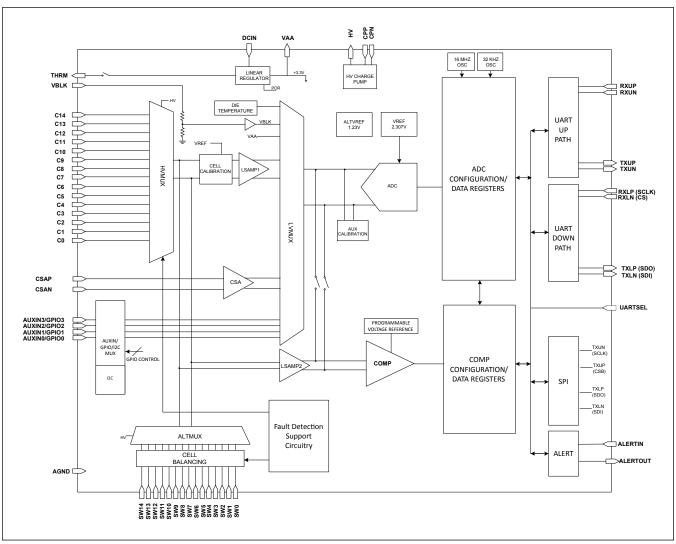
Figure 1. MAX17852 Functional Block Diagram
