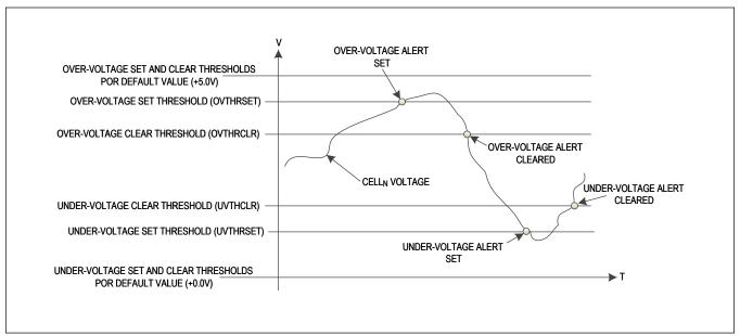
Figure 42. Cell Voltage-Alert Thresholds
