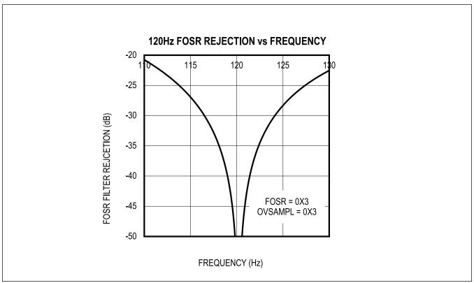
Figure 35. 120Hz Notch Filter
