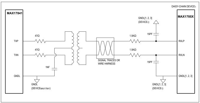
Figure 124. UART Transformer Isolation
