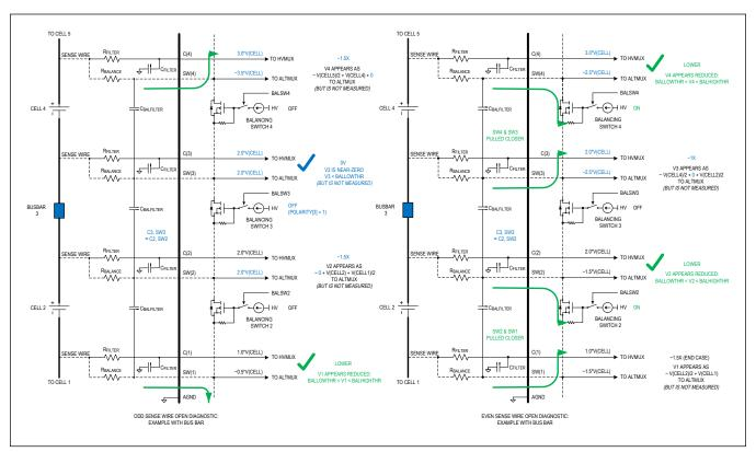
Figure 107. Cell Sense-Wire Open-Diagnostic Operations - (Normal Operation, Including Bus Bars)
