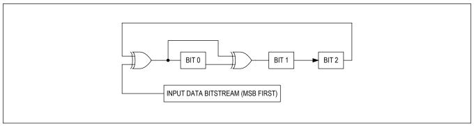
Figure 73. SPI CRC Calculation
