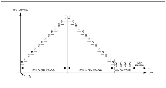
Figure 30. Comparator Single Scan With Oversampling
