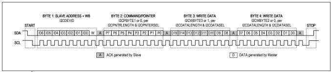
Figure 76. I<sup>2</sup>C Write Mode Transaction Example -- 7-Bit Address, I2C10BIT = 0
