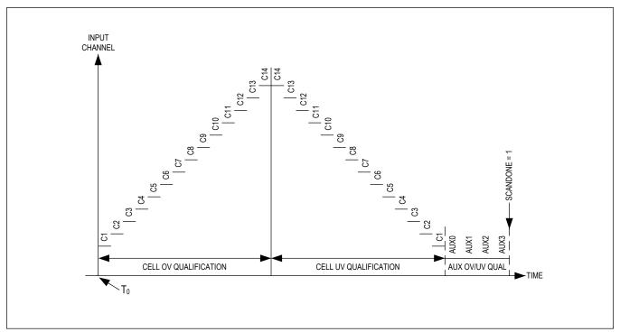
Figure 29. Comparator Single Scan Mode
