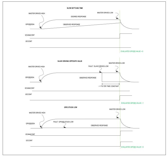
Figure 84. GPIO, I2CANACONT and I2CCONT timing diagram
