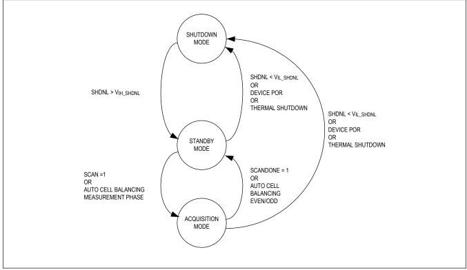
Figure 14. Operational Mode State Diagram
