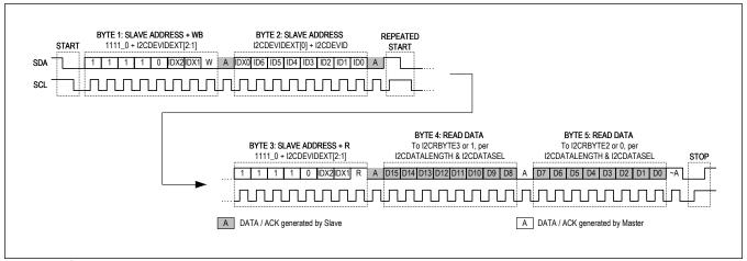
Figure 83. I<sup>2</sup>C Normal Format Read Mode Transaction Example -- 10-Bit Address, I2C10BIT = 1, I2CRFMT = 0
