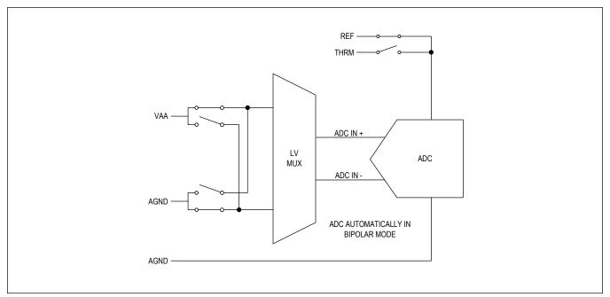
Figure 100. Full-Scale ADC Diagnostic Measurement
