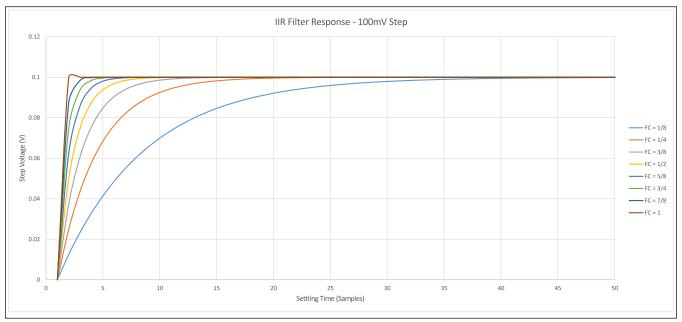
Figure 39. 100mV IIR Step Response
