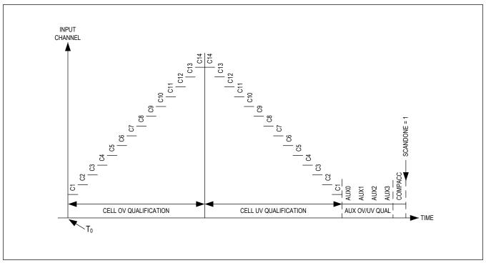
Figure 94. Comparator Accuracy End of Scan Measurement
