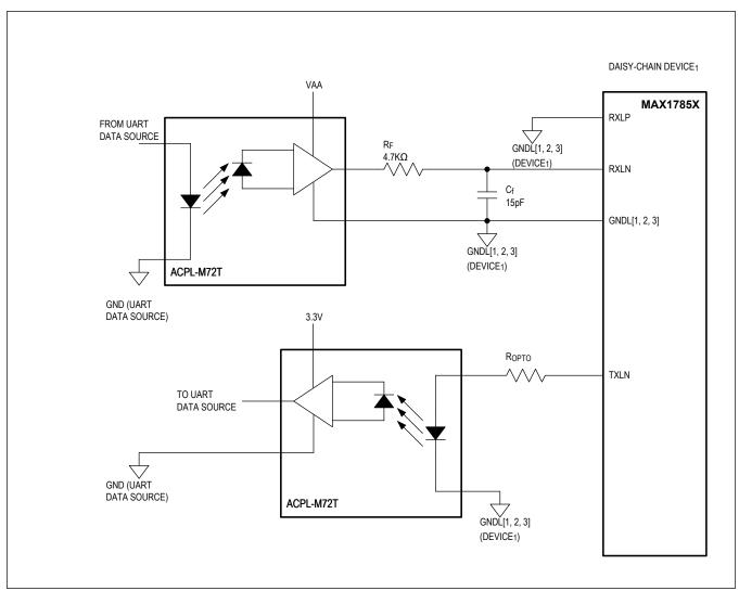
Figure 125. UART Optical Isolation
