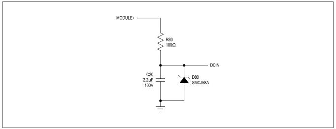
Figure 116. Power-Supply Connection
