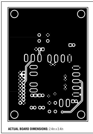
Figure 5. MAX1799 EV Kit PCB Layout—Solder Side
