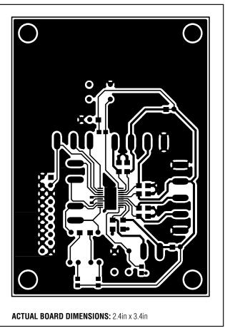
Figure 4. MAX1799 EV Kit PCB Layout—Component Side
