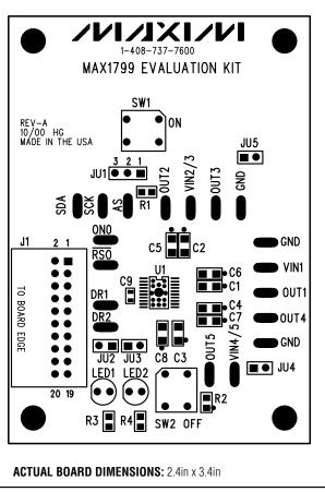
Figure 3. MAX1799 EV Kit Component Placement Guide— Component Side
