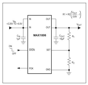
Figure 2. Adjustable Output Using External Feedback Resistors
