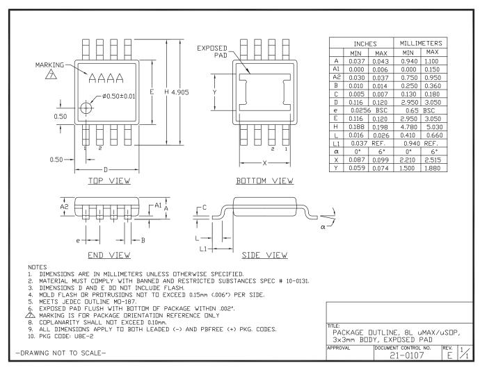
Note: The MAX1806 has on exposed thermal pad on the bottom side of the package.
