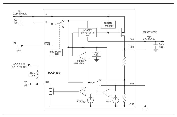
Figure 1. Functional Diagram
