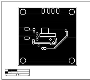
Figure 7. MAX1809 EV Kit PC Board Layout—Solder Side
