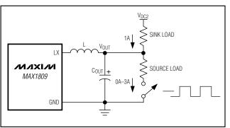
Figure 3. Load Transient Setup
