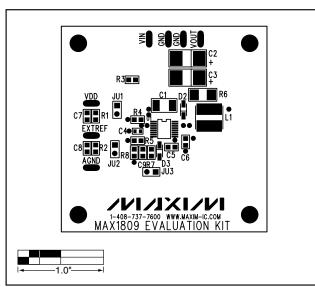
Figure 5. MAX1809 EV Kit Component Placement Guide— Component Side
