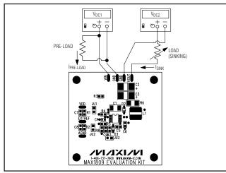
Figure 2. Test Setup (Sinking)
