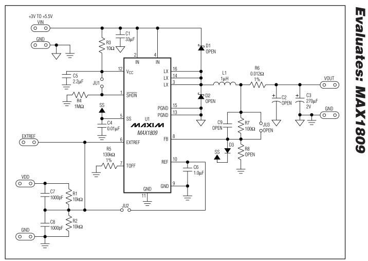
Figure 4. MAX1809 EV Kit Schematic
