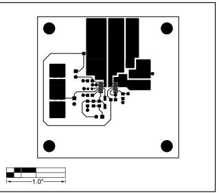
Figure 6. MAX1809 EV Kit PC Board Layout—Component Side
