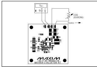
Figure 1. Test Setup (Sourcing)
