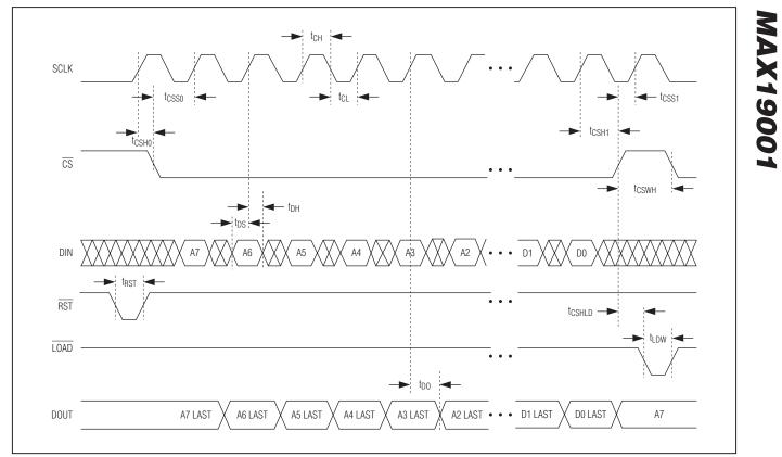
Figure 3. Detailed Serial-Port Timing Diagram
