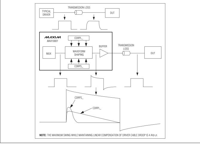
Figure 1. Driver Cable-Droop Compensation
