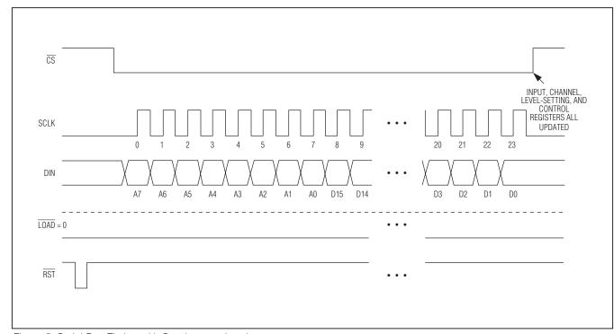
Figure 5. Serial-Port Timing with Synchronous Load
