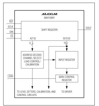
Figure 2. Serial-Interface Block Diagram
