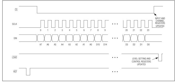
Figure 4. Serial-Port Timing with Asynchronous Load
