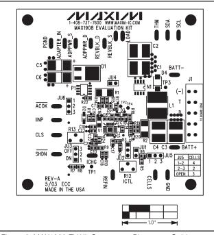
Figure 2. MAX1908 EV Kit Component Placement Guide—Component Side
