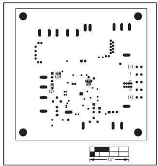
Figure 7. MAX1908 EV Kit PC Board Layout—Solder Side
