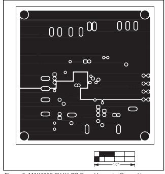
Figure 5. MAX1908 EV Kit PC Board Layout—Ground Layer
