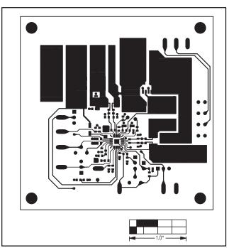
Figure 3. MAX1908 EV Kit PC Board Layout—Component Side
