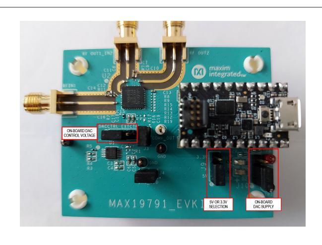
Figure 4. Connection Setup for Using On-Board Power Supply and On-Board Control Voltage
