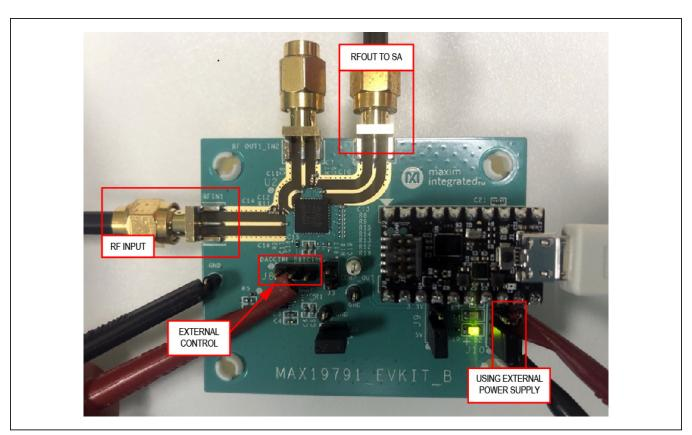
Figure 1. Connection Setup for Using External Power Supply and External Control Voltage
