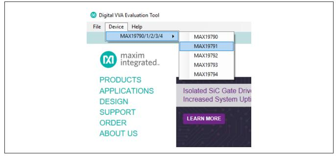
Figure 2. Part Selection in Common GUI
