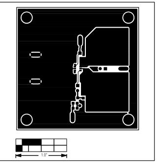
Figure 3. MAX1982 EV Kit PC Board Layout—Component Side
