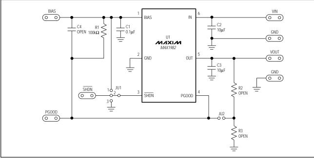
Figure 1. MAX1982 EV Kit Schematic
