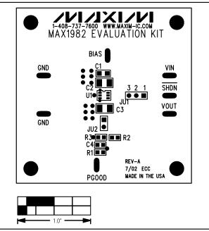
Figure 2. MAX1982 EV Kit Component Placement Guide— Component Side
