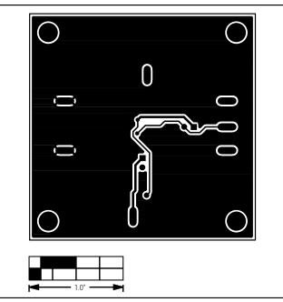
Figure 4. MAX1982 EV Kit PC Board Layout—Solder Side
