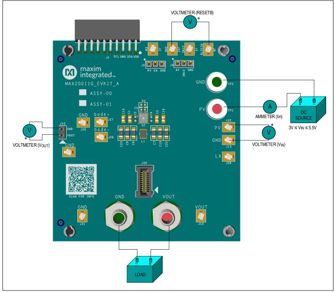
Figure 1. MAX20011G Evaluation Kit Configuration
