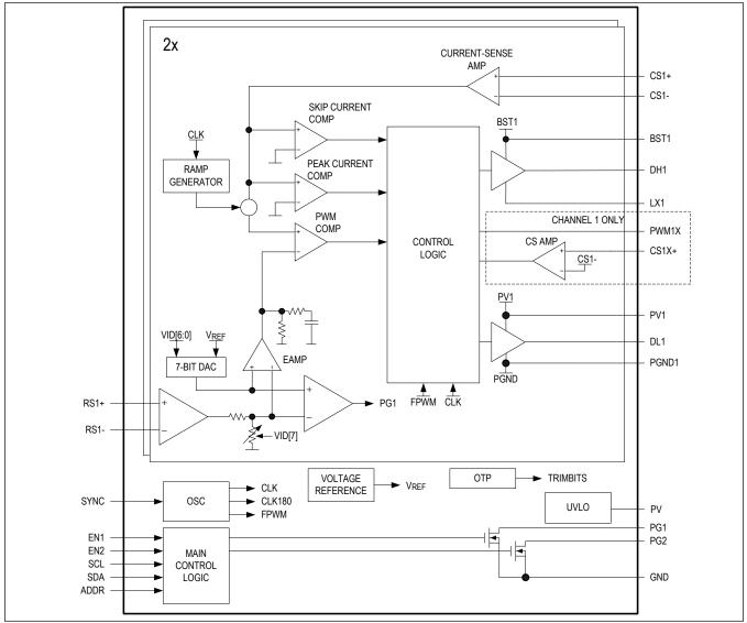
Figure 1. Internal Block Diagram
