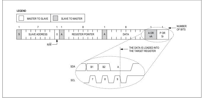
Figure 6. Write Byte Format
