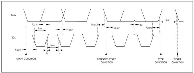
Figure 2. I<sup>2</sup>C Timing Diagram
