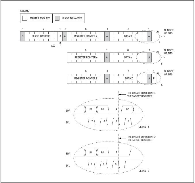
Figure 7. Write Register-Data Pair Format
