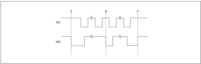
Figure 3. START, STOP, and Repeated START Conditions
