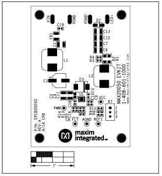
Figure 2. MAX20050 EV kit Component Placement Guide—Component Side
