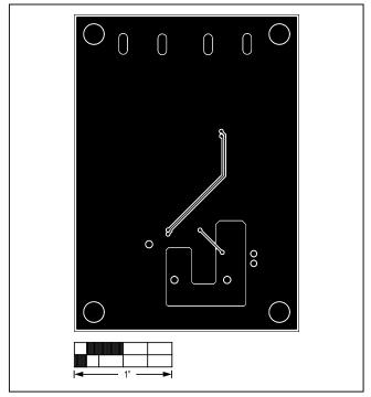
Figure 4. MAX20050 EV Kit PCB Layout—Solder Side
