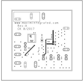
MAX20059 EV Kit Component Placement Guide—Bottom
