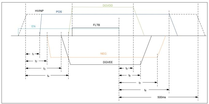
Figure 1. TFT Sequence with  $R_{SEQ} = 10k\Omega$
