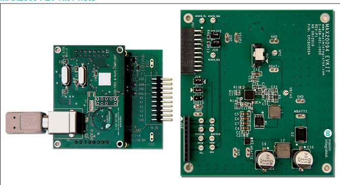
Note: Photo shows the Maxim MINIQUSB board on left and the MAX20094 EV kit board on right.
