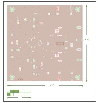
Figure 4. MAX20097 EV Kit PCB Layout—Inner Layer 1
