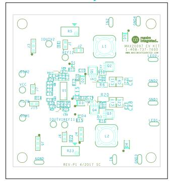
Figure 2. MAX20097 EV Kit Component Placement Guide—Component Side
