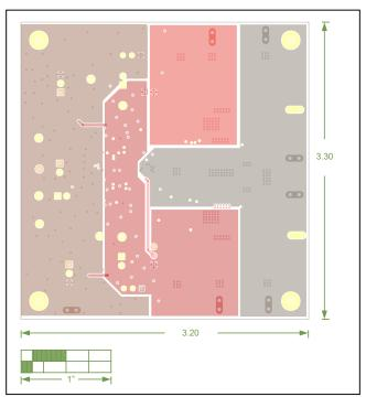
Figure 6. MAX20097 EV Kit PCB Layout—Bottom Layer
