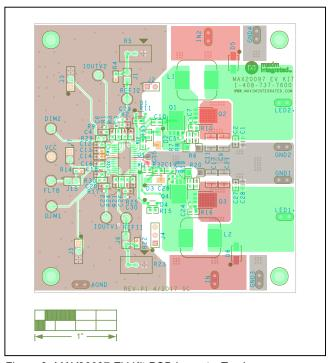
Figure 3. MAX20097 EV Kit PCB Layout—Top Layer
