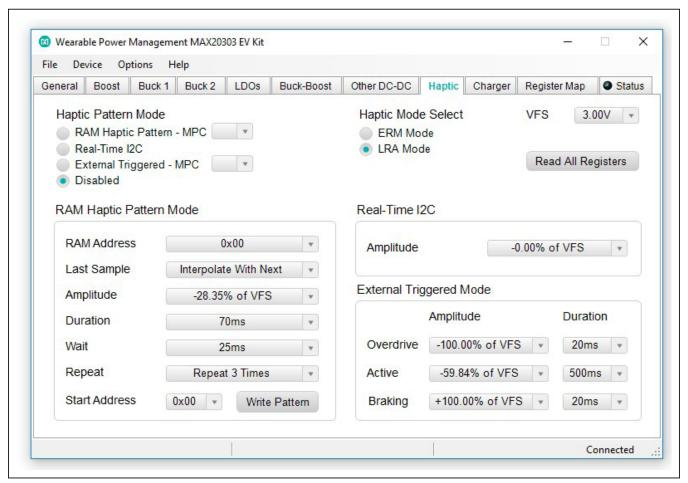
Figure 11. Haptic Tab
