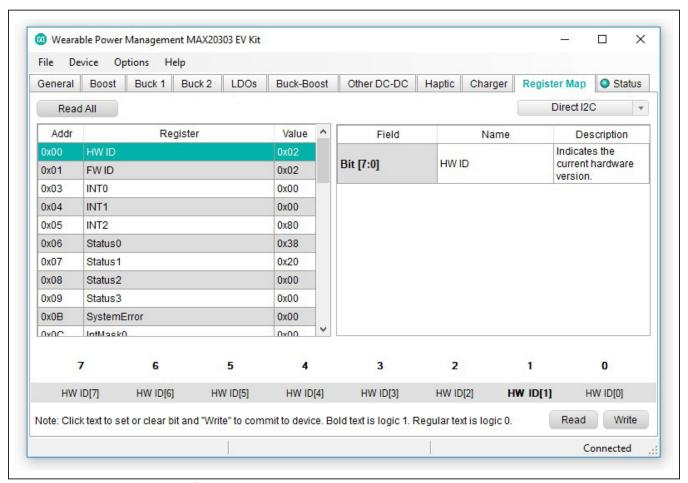
Figure 13. Register Map Tab Direct I<sup>2</sup>C
