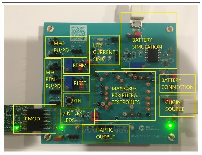
Figure 16. MAX20303 EVSYSKIT Block Annotated Picture
