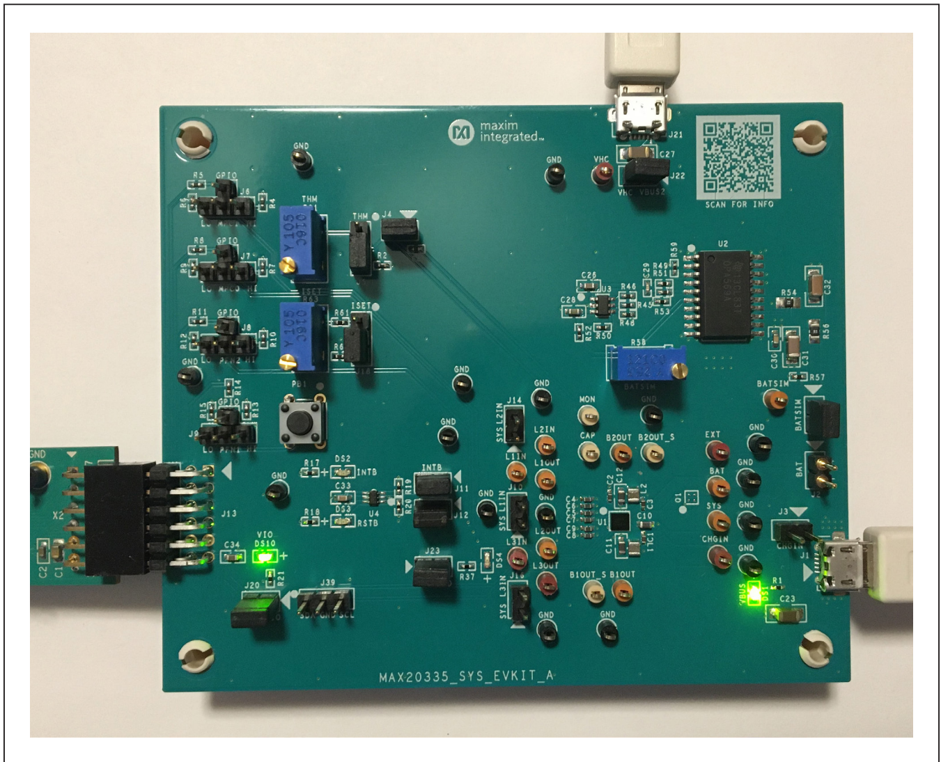
Figure 10. MAX20335 EV System Board Picture
