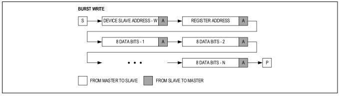
Figure 12. Burst Write Sequence
