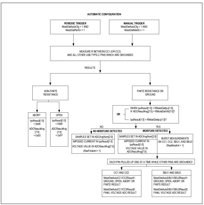
Figure 2. Automatically Configured Moisture Detection Flow
