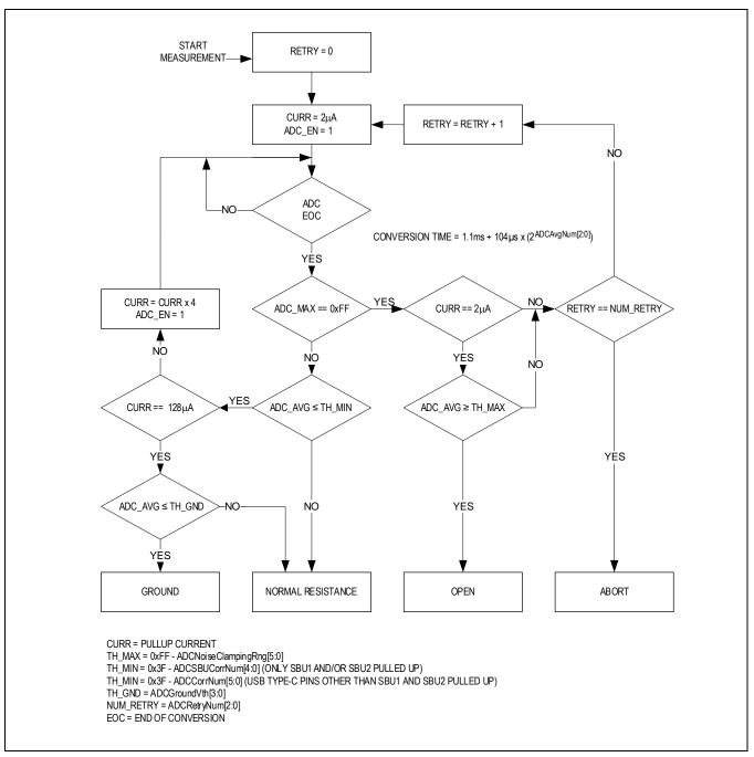
Figure 8. Resistive Measurement Flow
