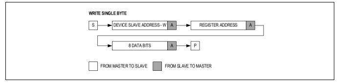
Figure 11. Write Byte Sequence
