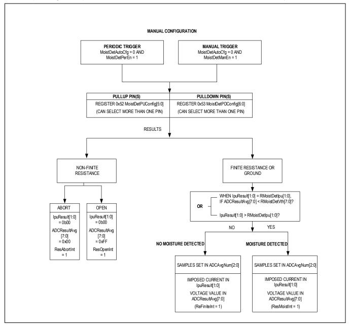
Figure 3. Manually Configured Moisture Detection Flow
