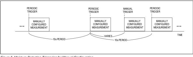
Figure 5. Moisture Detection Triggering for Manual Configuration
