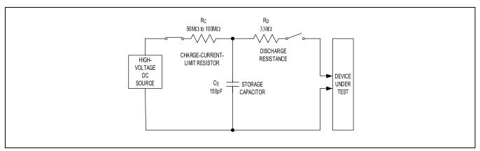
Figure 18. IEC61000-4-2 ESD Test Model
