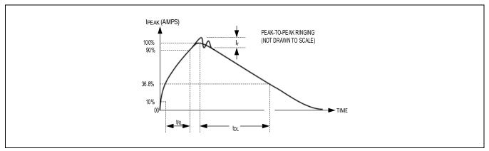
Figure 17. Human Body Current Waveform
