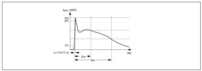
Figure 19. IEC61000-4-2 ESD Generator Current Waveform
