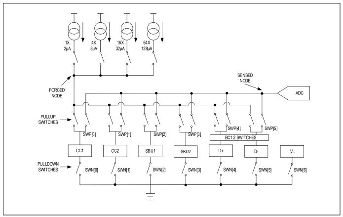
Figure 7. Resistive Measurement Simplified Diagram
