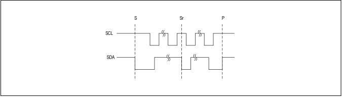
Figure 10. PC START, STOP, and REPEATED START Conditions
