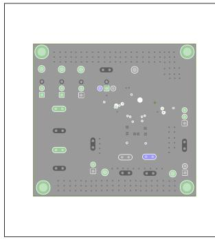
MAX20457 EV Kit PCB Layout - Internal Layer 2
