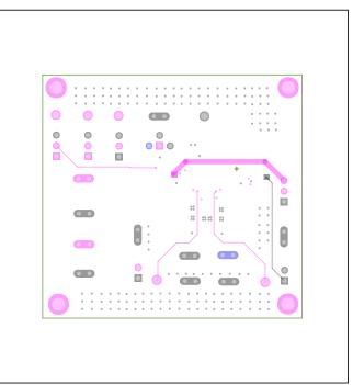
MAX20457 EV Kit PCB Layout - Internal Layer 3
