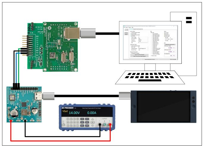
Figure 3. I<sup>2</sup>C EV Kit Setup
