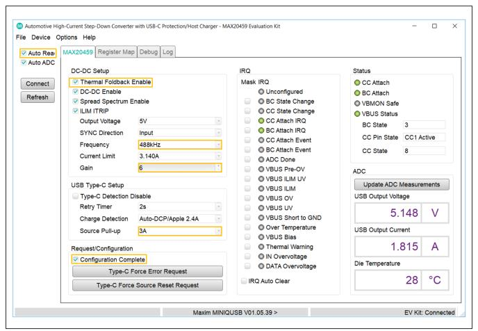
Figure 5. MAX20459 GUI Configured
