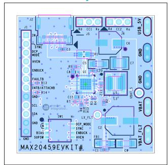
MAX20459 EV Kit PCB Layout - Top View
