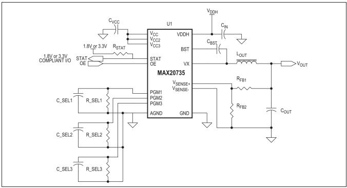
Figure 3. Typical Application Circuit
