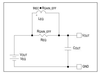
Figure 4. Averaged Small-Signal Equivalent Circuit of Regulator
