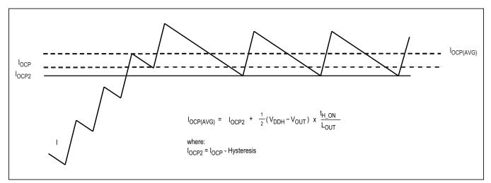
Figure 2. Inductor Current During Current Limiting
