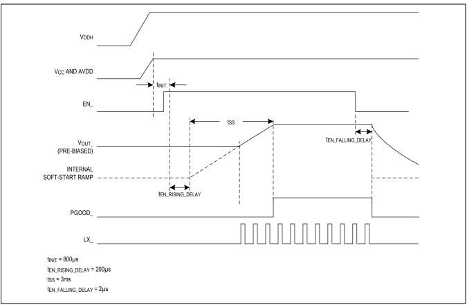
Figure 3. Startup and Shutdown Timing
