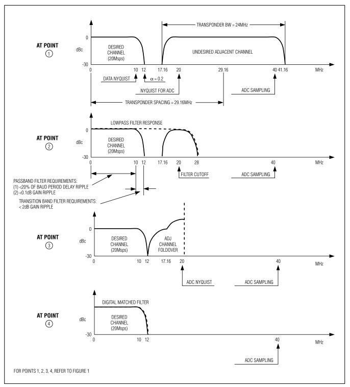
Figure 2. Lowpass Filtering Example
