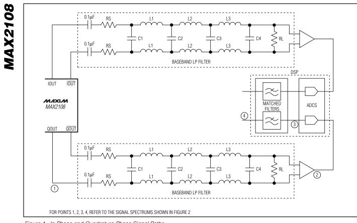
Figure 1. In-Phase and Quadrature-Phase Signal Paths
