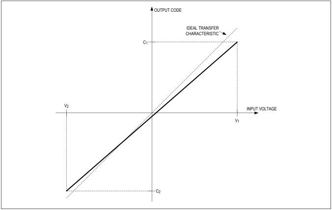
Figure 11. Definition of Parameters for Two-Point Calibration
