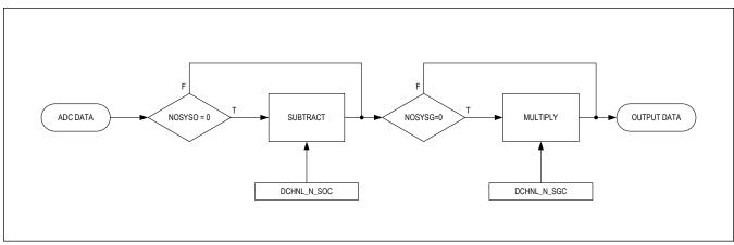
Figure 10. ADC System Calibration Data Flow
