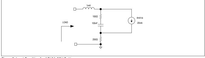
Figure 3. Load Condition for AOVM, 25V Setting
