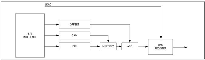
Figure 4. Gain and Offset Adjustment
