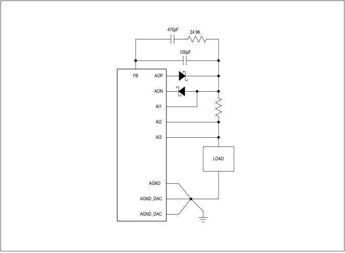
Figure 7. Recommended Compensation Network
