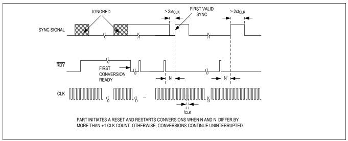
Figure 9. SYNC Input Timing
