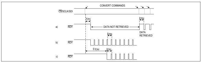
Figure 8. RDY Output Timing, a) Single-Cycle Mode, b) Continuous Single-Cycle Mode, c) Continuous Conversion Mode
