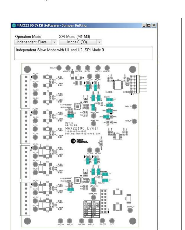
Figure 7. MAX22190 EV Kit Software—Jumper Setting Diagram
