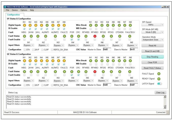
Figure 4. MAX22190 EV Kit Software—Read DI Continuously
