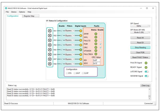
Figure 3. MAX22199 EV Kit Software—Read DI Continuously
