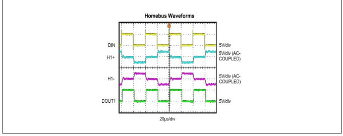
Figure 1. MAX22288 EV Kit Waveforms at 50kbps
