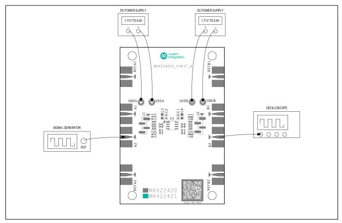
Figure 3. MAX22421BS EV kit typical test setup
