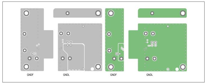
Figure 10. Stitching Capacitance on Internal Layers
