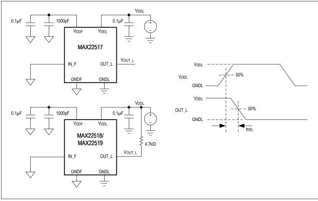
Figure 2. Power-Up Delay Timing Diagram
