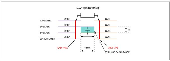
Figure 9. Stitching Capacitance Example on a 4-Layer PCB
