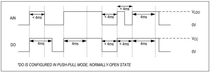
Figure 3. Sample Waveform with Positive Pulse Stretching
