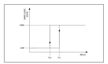
Figure 2. Comparator Operation with Hysteresis
