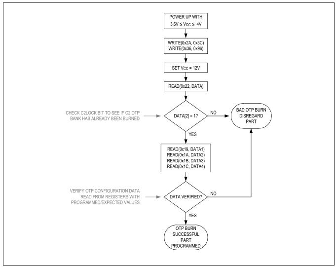
Figure 12. Bank C2 OTP Configuration Check
