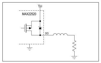
Figure 4. High-Side Mode with Ground-Connected Load
