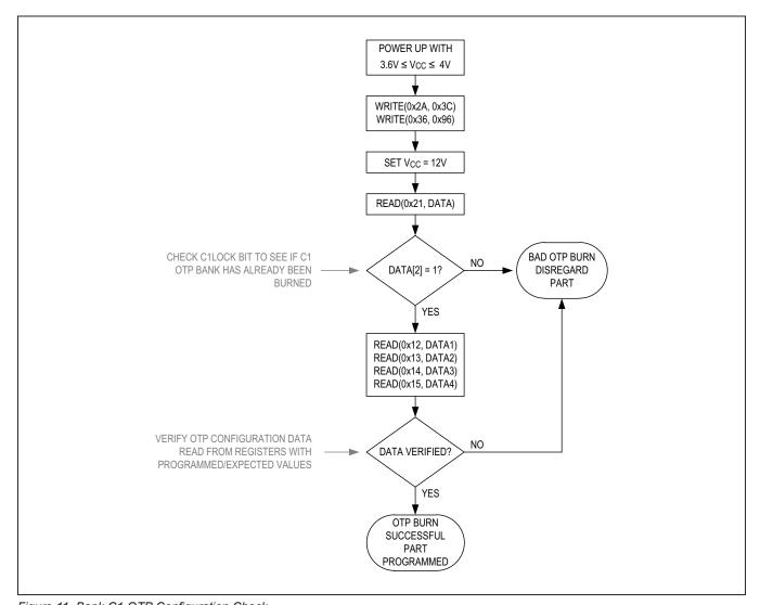
Figure 11. Bank C1 OTP Configuration Check
