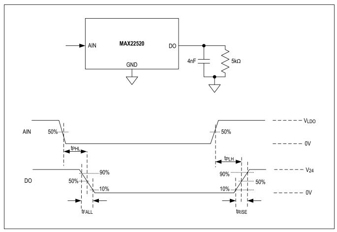
Figure 1. DO Driver Propagation Delays (Push-Pull Mode)
