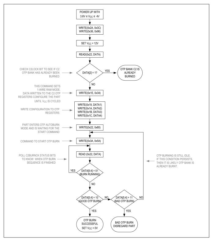
Figure 10. Bank 2 OTP Configuration Flow Chart
