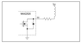
Figure 5. Low-Side Mode with Supply-Connected Load
