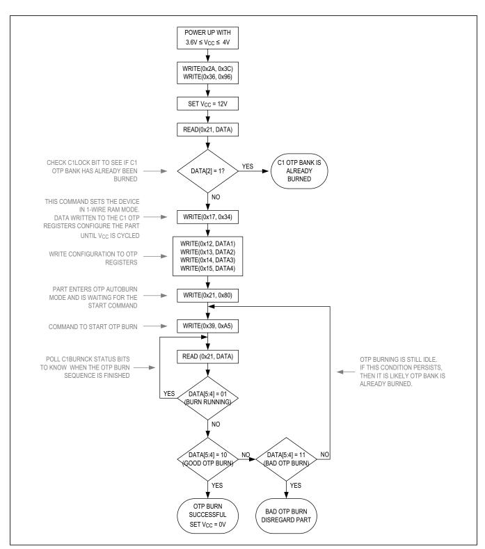
Figure 9. Bank 1 OTP Configuration Flow Chart
