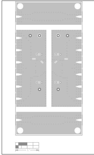
MAX22563-MAX22566 EV Kit PCB Layout—Layer 2 GND
