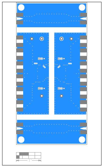
MAX22563–MAX22566 EV Kit PCB Layout—Bottom Layer
