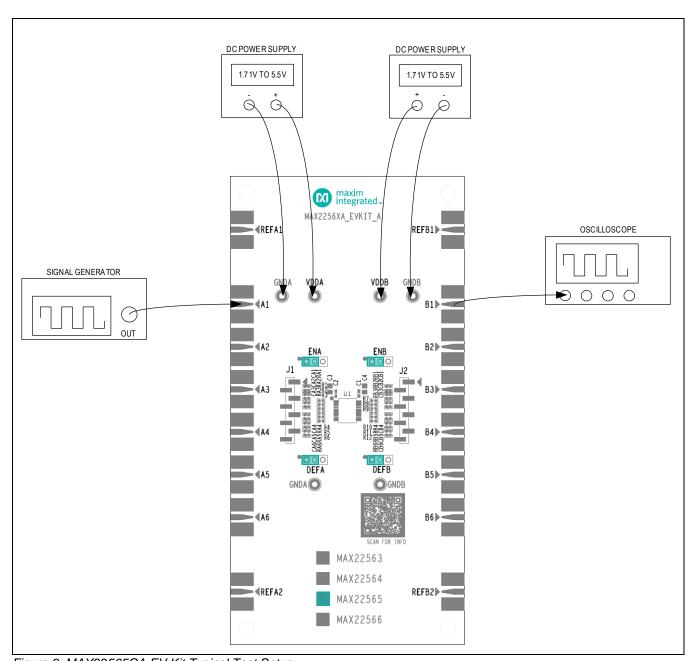
Figure 3. MAX22565CA EV Kit Typical Test Setup
