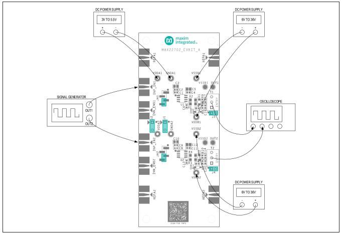
Figure 3. MAX22701 and MAX22702 EV Kits Typical Test Setup
