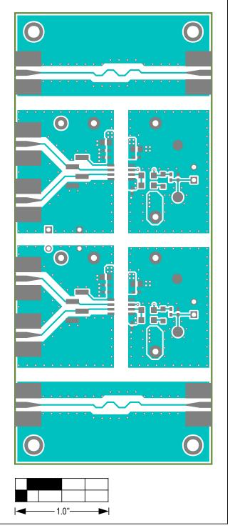
MAX22701 EV Kit PCB Layout—Top View
