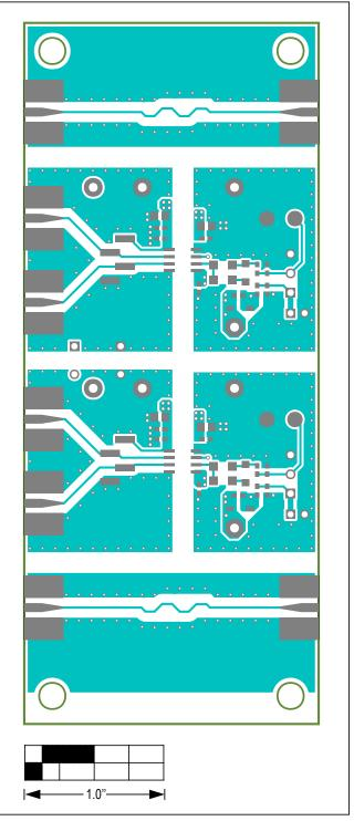
MAX22702 EV Kit PCB Layout—Top View
