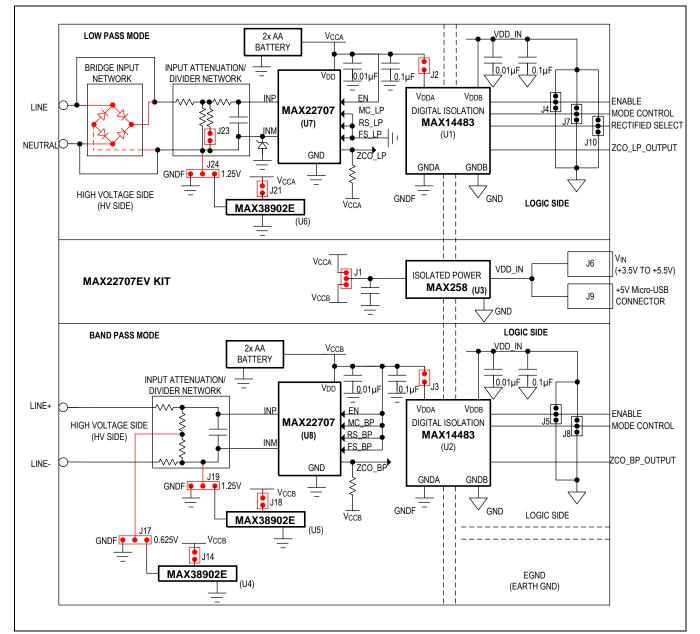
Figure 1. MAX22707EV Kit High Voltage Test Configuration
