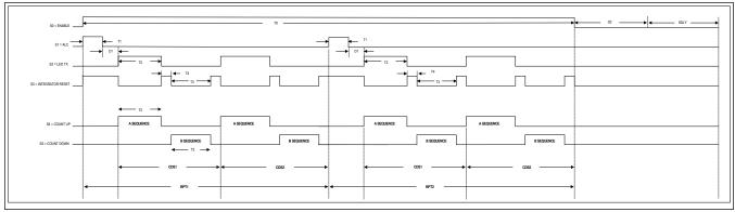
Figure 1. Timing Setting: NCDS = 2, NRPT = 2, CRST = 1
