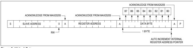
Figure 6. Write 1 Byte
