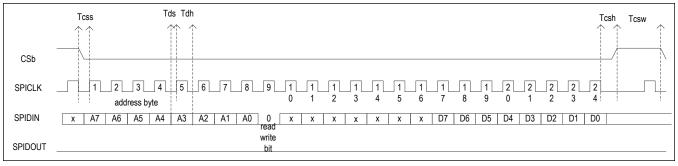
Figure 10. SPI Write
