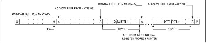
Figure 7. Write n Bytes
