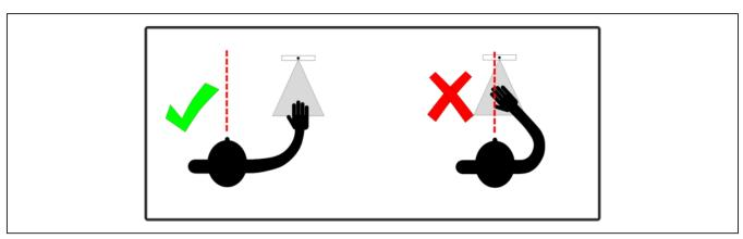
Figure 5: Correct Sensor Position, Directed to Side of Body
