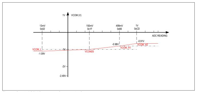
Figure 4. Sample VCOM Temperature Compensation Curve
