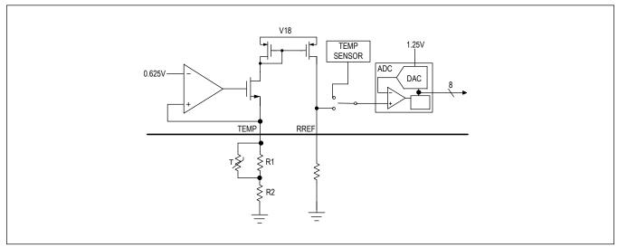
Figure 2. Possible NTC Connection
