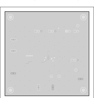
MAX25232 EV Kit PCB Layout—Internal Layer 2
