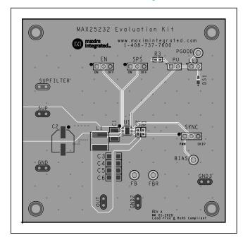
MAX25232 EV Kit Component Placement Guide—Top View
