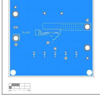
MAX25262/MAX25263 EV Kit PCB Layout — Internal Layer 3
