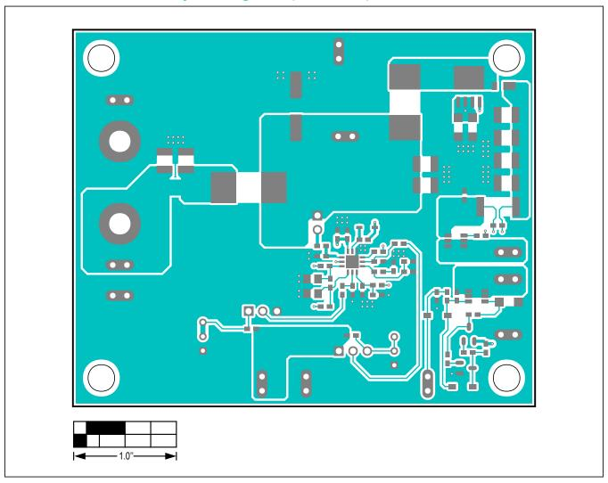
MAX25611 EV Kit PCB Layout—Top View
